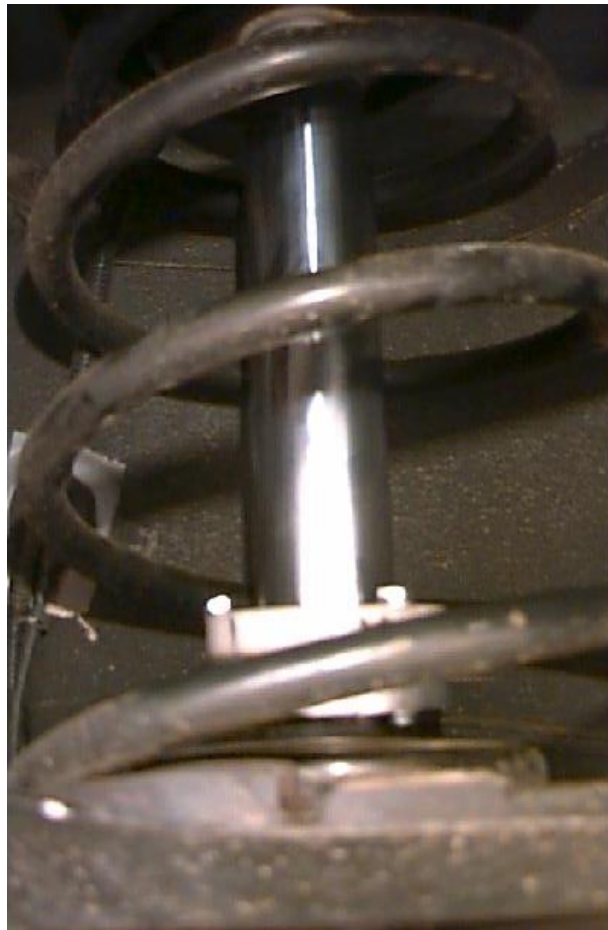
Figure 5.6. Physical Installation of MR Damper
