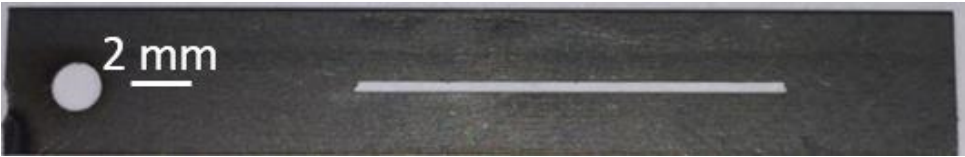
Figure 33: Extractor machined on stainless steel with a 500 μm slot
