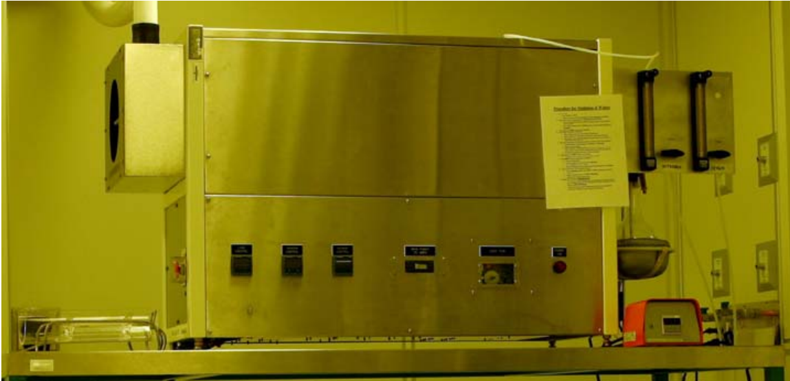
Figure 26 Side control panel of oxidation furnace.
