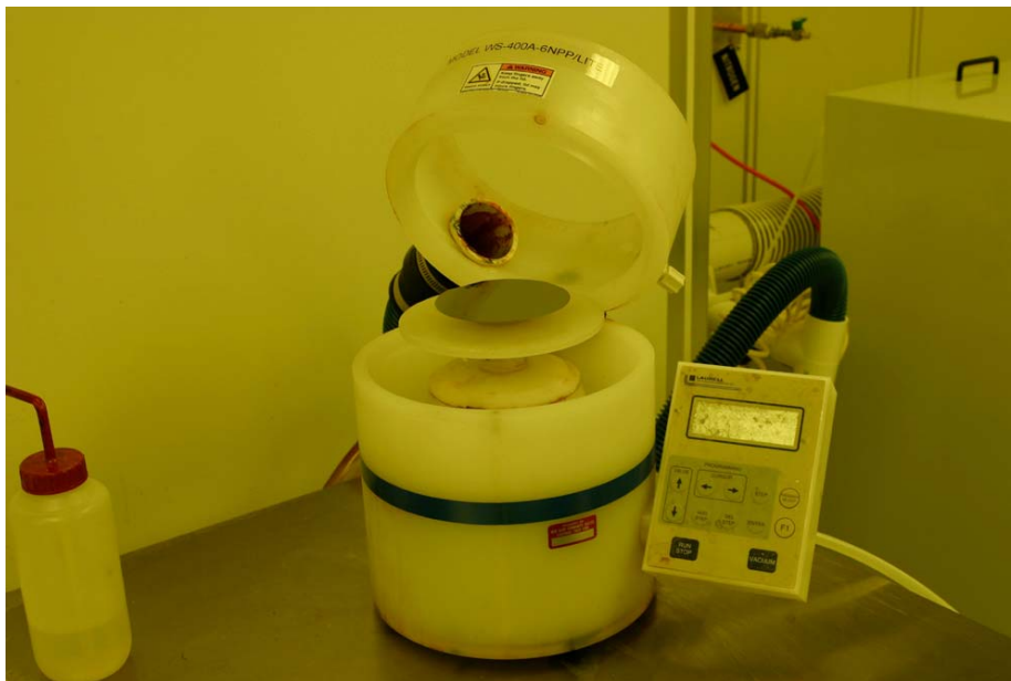
Figure 31 Laurell Spin Coater. Used to spin photoresist, spin-on boron, and to clean the wafers with acetone and IPA.
