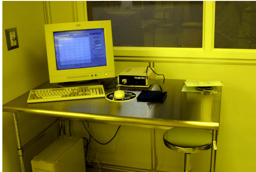
Figure 32 Filmetrics F20 Thin-Film Measurement System. Used in the VTPMOS process to measure oxide thicknesses.
