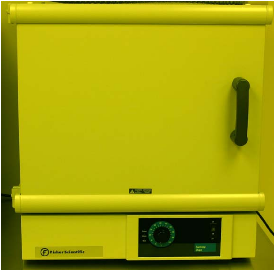
Figure 34 Convection oven used in boron predeposition.
