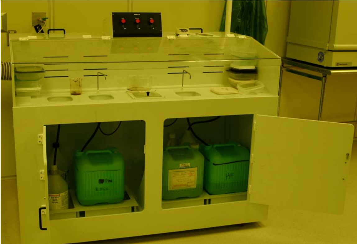
Figure 36 Wet bench. Left side accommodates photoresist developer and solvents. Right side accommodates HF.
