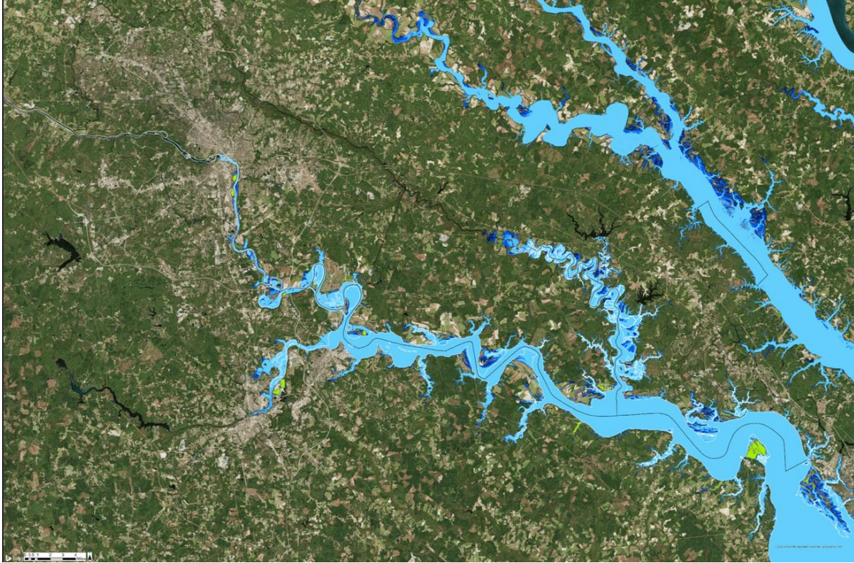
Figure 15. Sea-level rise map in 2100 along the James River. Light blue indicates the highly likely scenario of 1-3ft, while the dark blue indicates the possible scenario of 3-6ft. Green showcases low-lying land that will flood.
