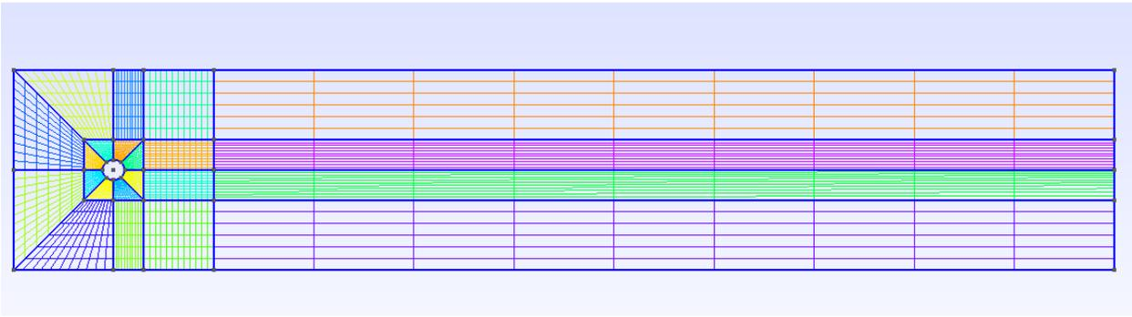
Figure B.8: Fine wide elliptical cylinder mesh generated in Gmsh for shape optimization cases.
