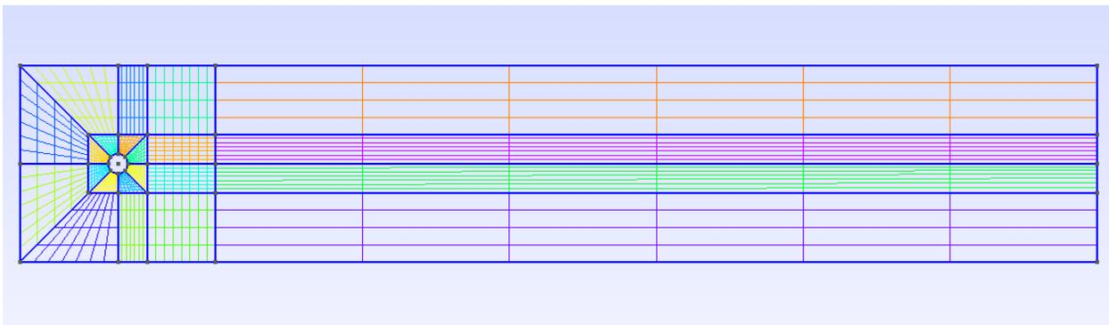
Figure B.2: Medium circular cylinder mesh generated in Gmsh for shape optimization cases.
