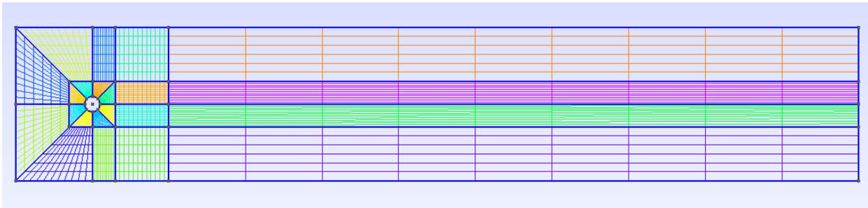
Figure B.3: Fine circular cylinder mesh generated in Gmsh for shape optimization cases.
