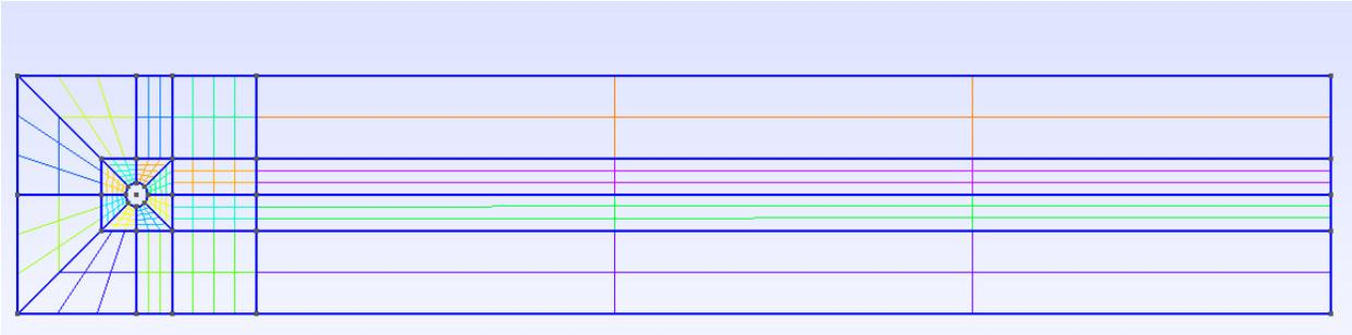
Figure B.11: Coarse narrow elliptical cylinder mesh generated in Gmsh for shape optimization cases.
