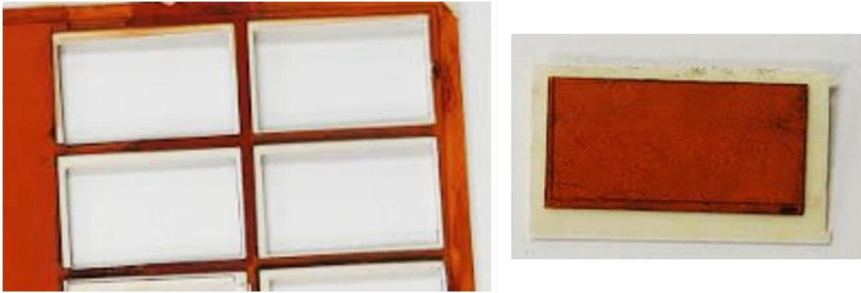
Figure 6. To reduce ceramic cracking during cutting, traces were left between sample cutouts (right) and a backplane was added to the back of each sample (left)
