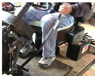
Figure 8. Modified tractor controls for operators with disabilities: (upper left) tractor controls on the right to accommodate a left-hand amputee; (upper right) spinner knob for steering wheels for better grip and one-hand steering; (lower) hand levers for brake engagement for limited leg mobility or strength.
