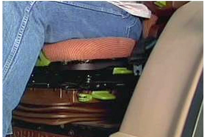
Figure 1. Improved seat suspensions or custom-fitted seats will isolate the operator from low-frequency vibration.
