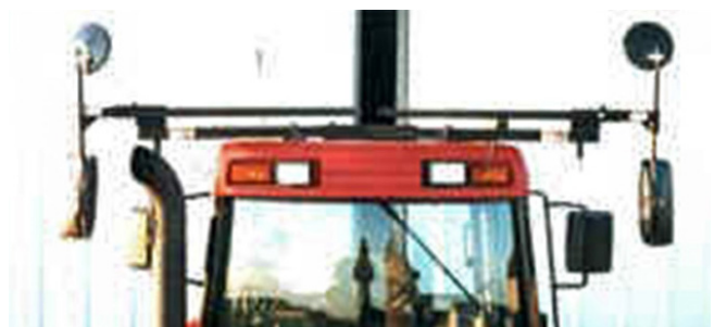
Figure 10. Extra, enlarged, or extended mirrors to reduce neck and back strain.
