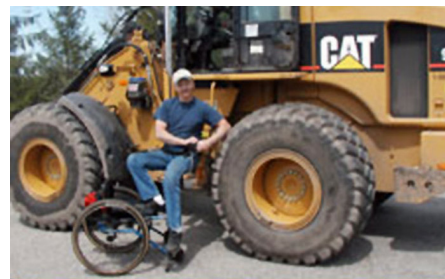
Figure 5. Mechanical lift used for accessing the tractor operator's platform.
