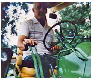
Figure 8. Modified tractor controls for operators with disabilities: (upper left) tractor controls on the right to accommodate a left-hand amputee; (upper right) spinner knob for steering wheels for better grip and one-hand steering; (lower) hand levers for brake engagement for limited leg mobility or strength.
