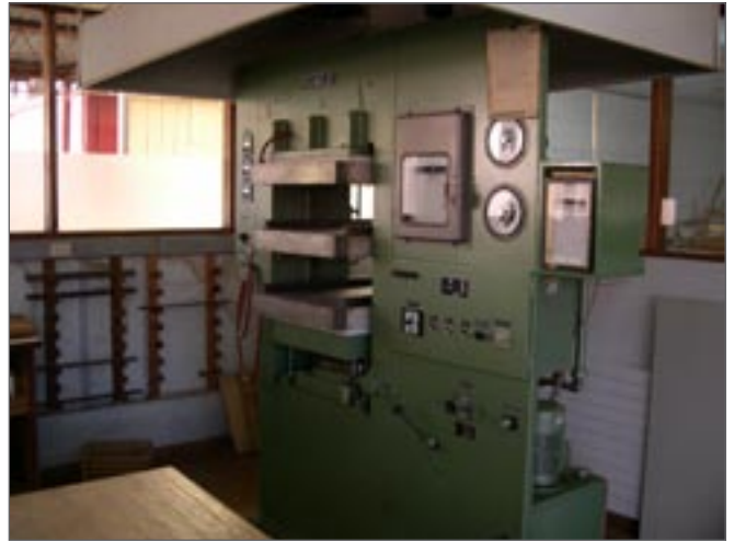
Laboratory hot press with two openings and electrically heated platens at the University of Austral.
