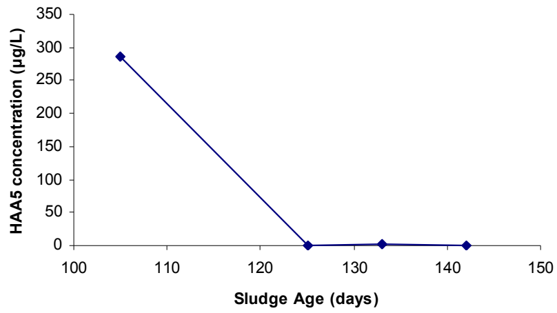
FIGURE 3 Sludge Age and HAA5 concentrations in centrifuged bottom samples
