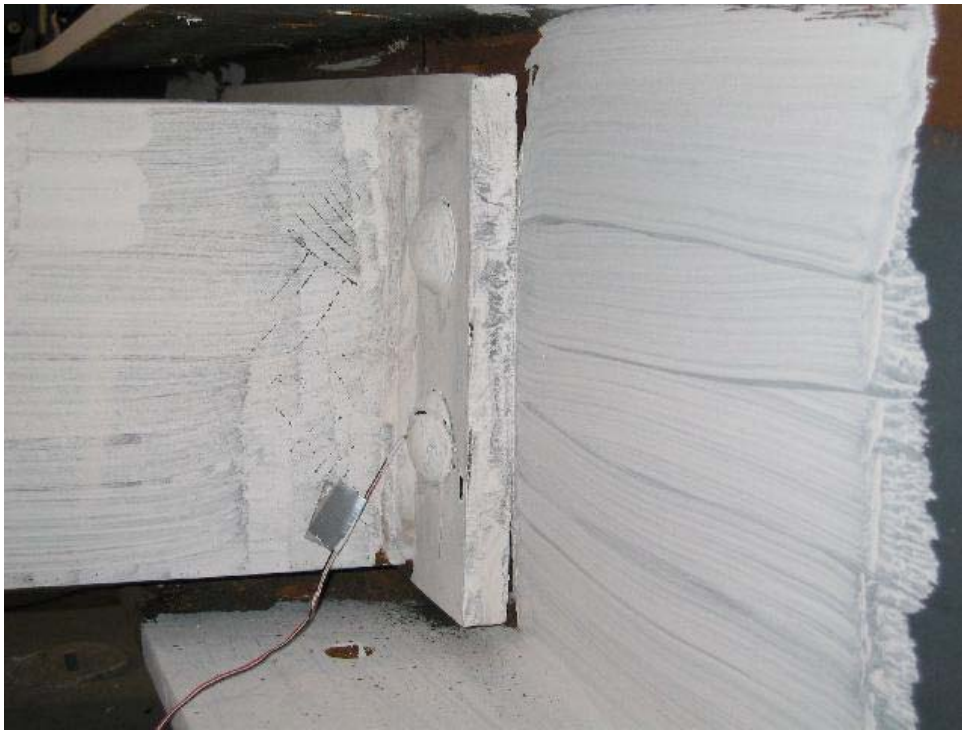
FIGURE 3.4: END-PLATE SEPARATION AND COLUMN WEB DISTORTION, TEST W27x84
