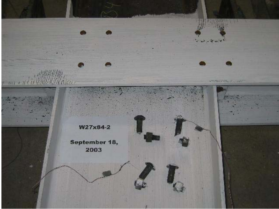
FIGURE 3.5: BOLT RUPTURE AT END OF TEST W27x84
