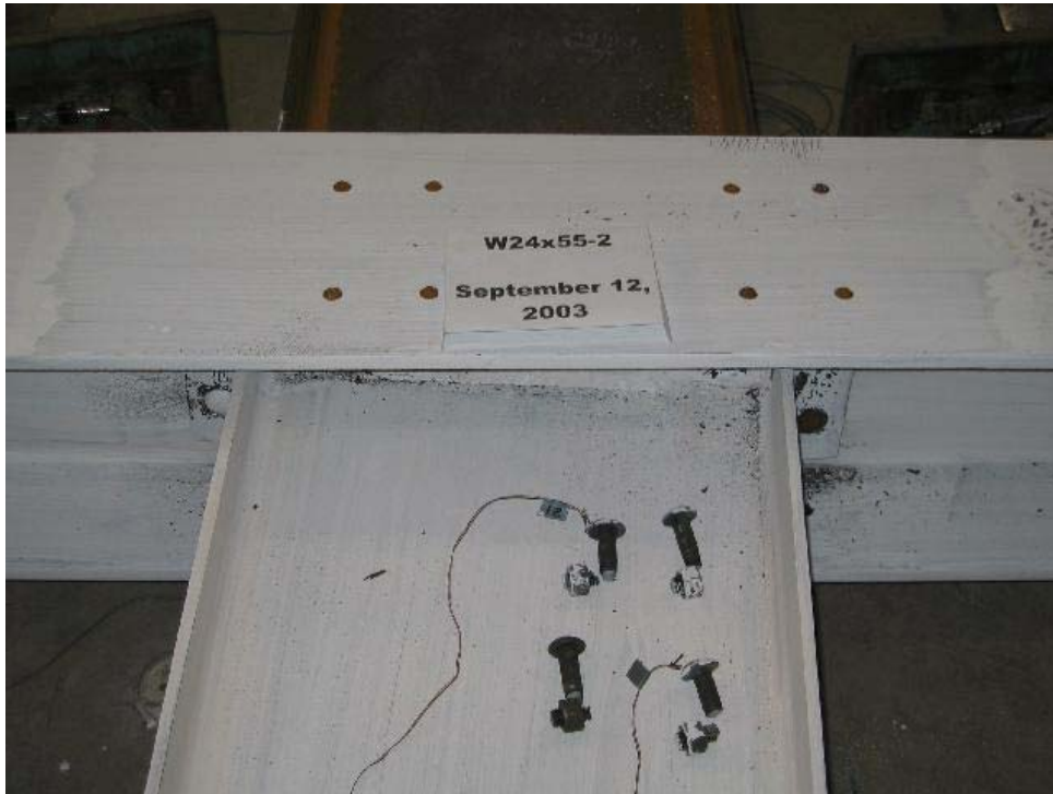
FIGURE 3.2: BOLT RUPTURE AT END OF TEST W24x55
