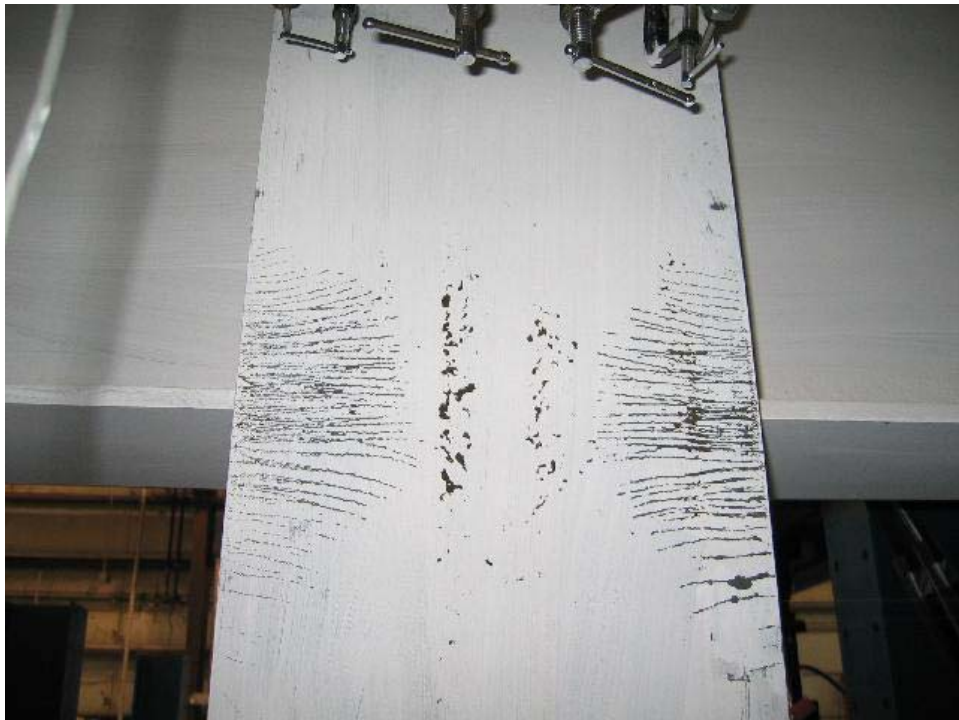
FIGURE 3.10: WHITEWASH FLAKING ON NORTH COLUMN FLANGE AFTER COMPLETION OF LOAD SEQUENCE #5
