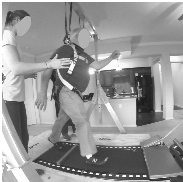
Figure 1. Photograph of a participant performing a reactive balance test. Visible is the harness and overhead gantry that prevented falls in the event of an unsuccessful test, and spotters on either side of the resident.
