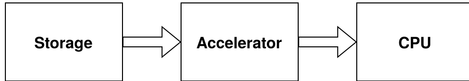
Figure 8.3: This design is based on Near-Data-Computation, where the accelerator is directly attached to the storage in-the-data-path. Any logic offloaded from the host system to the accelerator results in input data fetched into the accelerator’s memory and processed before reaching the host system’s main memory.
