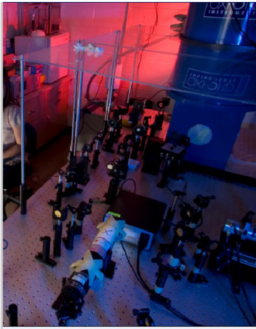
Figure 4.9: Our setup; showing magnet (top right), outside sample (top center), chopper (left), waveplates (center), and balanced detector for MOKE (right)
