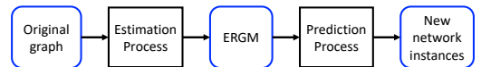
Fig. 2: The ERGM graph generation process where a network instance (at left) is used to estimate an ERGM (center). This model is then used to predict (generate) new graph instances (at right) that are similar to the original graph.
