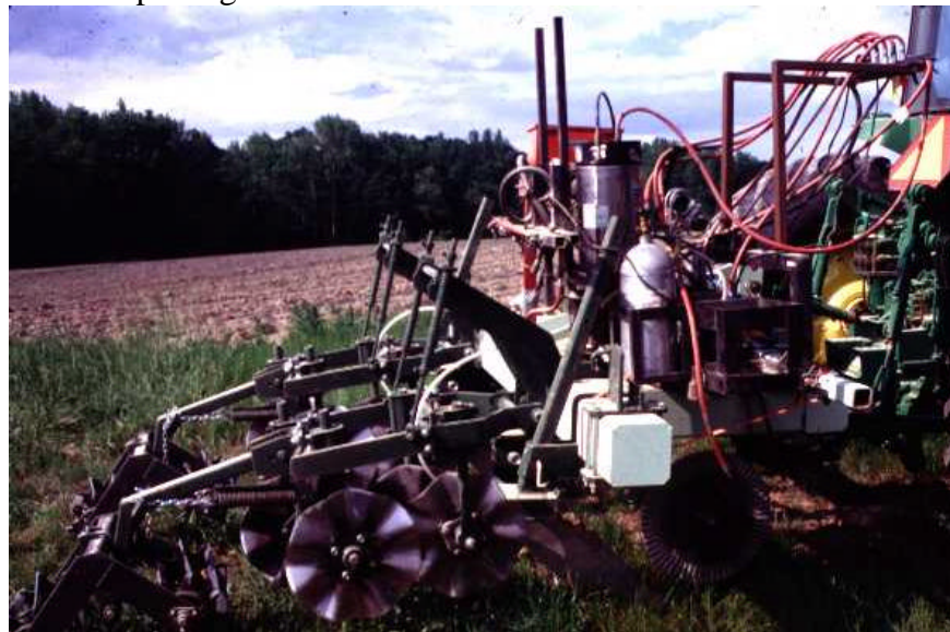
Figure 3.2. CO 2 -powered delivery system for injection of starter fertilizer in strip-tillage.
