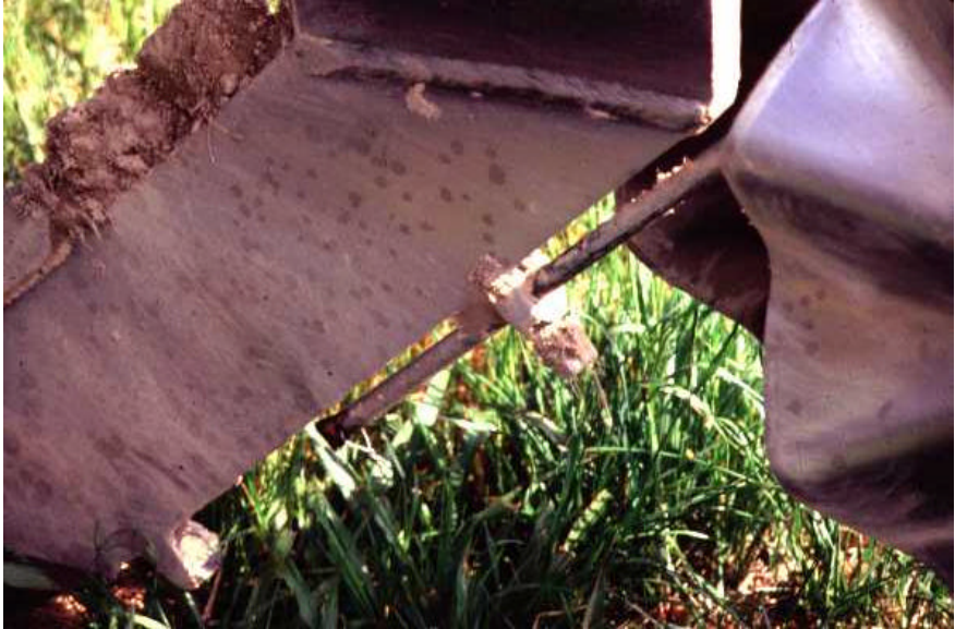
Figure 3.1. A modified sub-soil shank with 0.95 cm stainless steel fumigation tube attached for injection of starter fertilizer.
