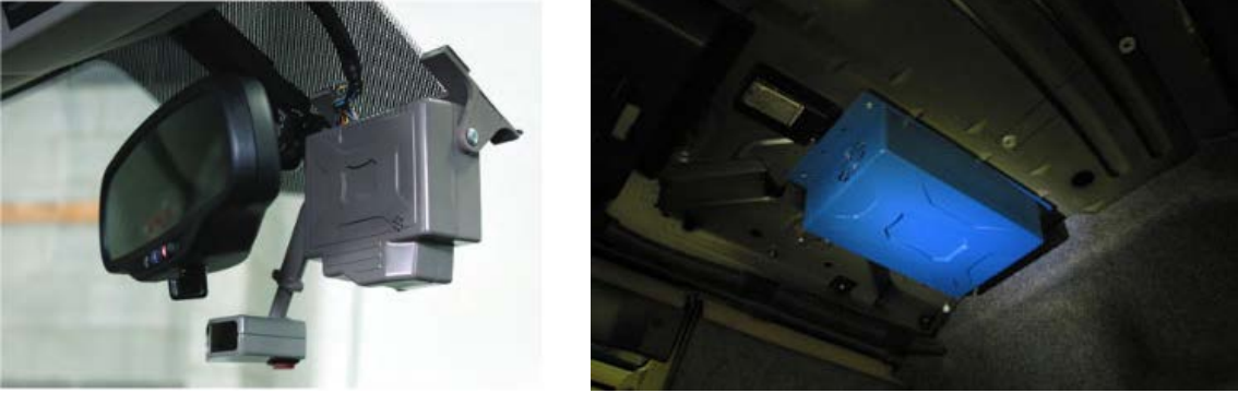
Figure 2. Photos. SHRP 2 NDS DAS installation showing head unit located behind the rearview mirror (left) and the main unit mounted to top of trunk (right).
