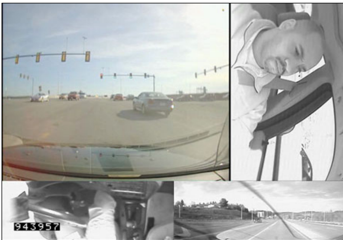
Figure 1. Photo. SHRP 2 NDS type video views showing forward, face, hands, and rear camera views (non-participant shown in photo).
