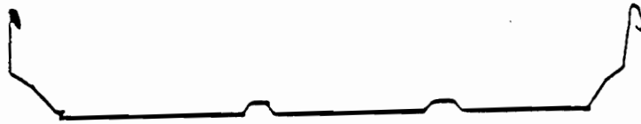
a) Typical Rib Type Panel
