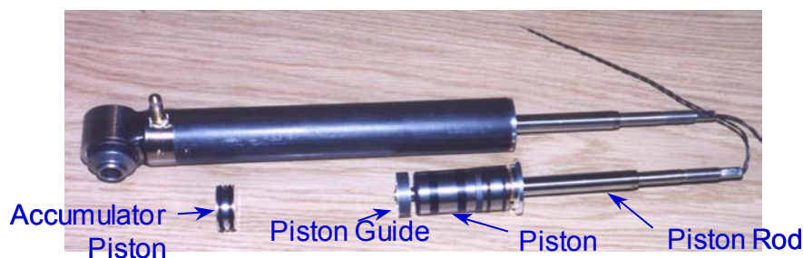
Figure 2-4. Disassembled MR Damper [53]
