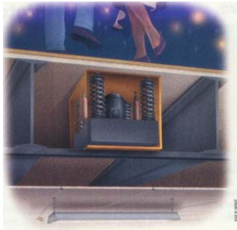
Figure 1-1. Correcting Human-Induced Floor Vibration Problems [4]
