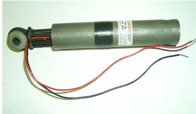
Figure 5-7. The Magneto-Rheological Sponge Damper for Semiactive Tuned Vibration Absorber
