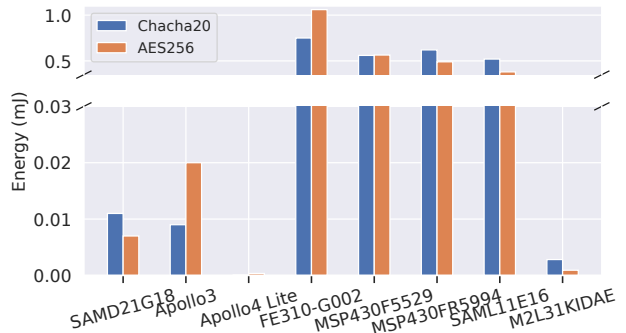
Figure 3: Energy consumption of symmetric-key encryption across devices.
