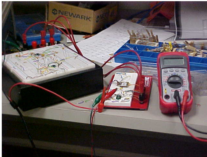
Figure B-4. Testing of line driver involves measuring the current with a multimeter.
