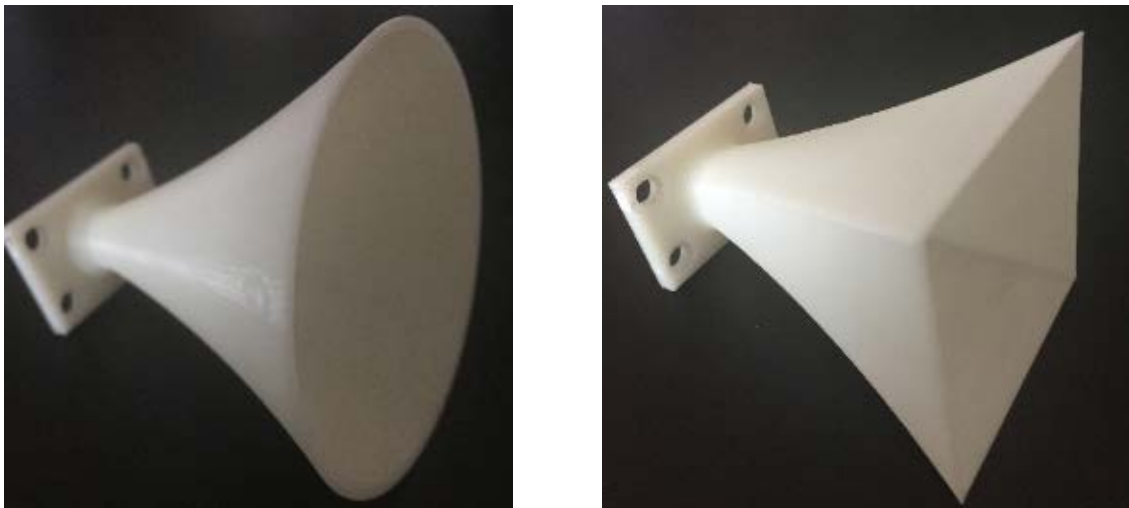
Figure A8: New acoustic horns additively manufactured as candidates for the dual Hartmann generator: Exponential with circular cross-section (left) and exponential with rectangular cross-section (right)
