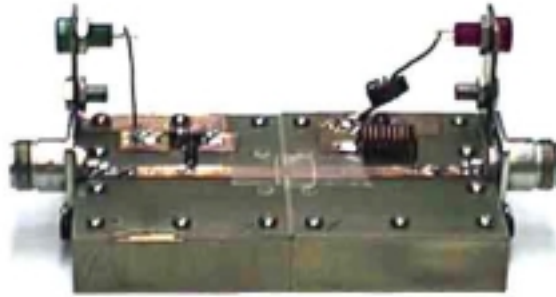
Figure 3.9. Break-apart fixture setup for measuring the thru standard.
