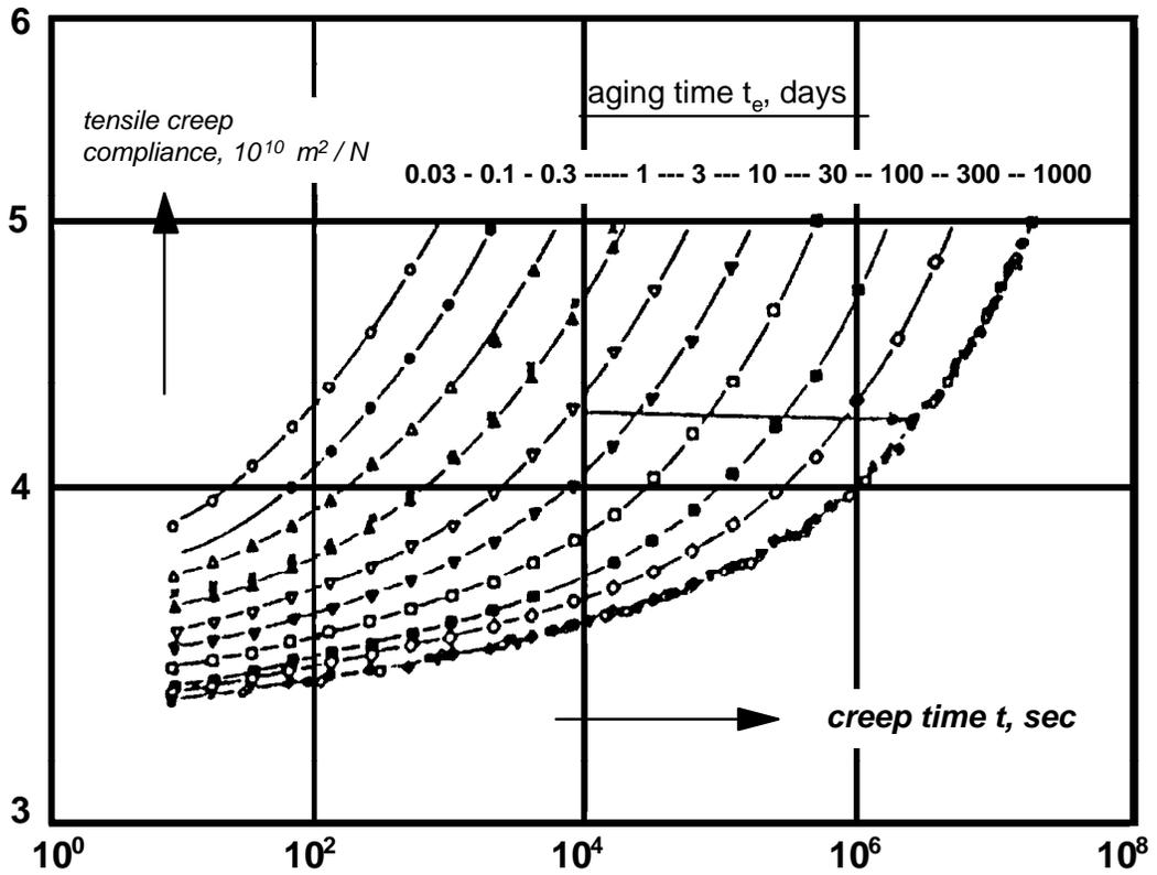
**Figure 2-4.** Small strain tensile creep curves of rigid PVC quenched from 90°C to 40°C and annealed at 40°C. (69,70)
