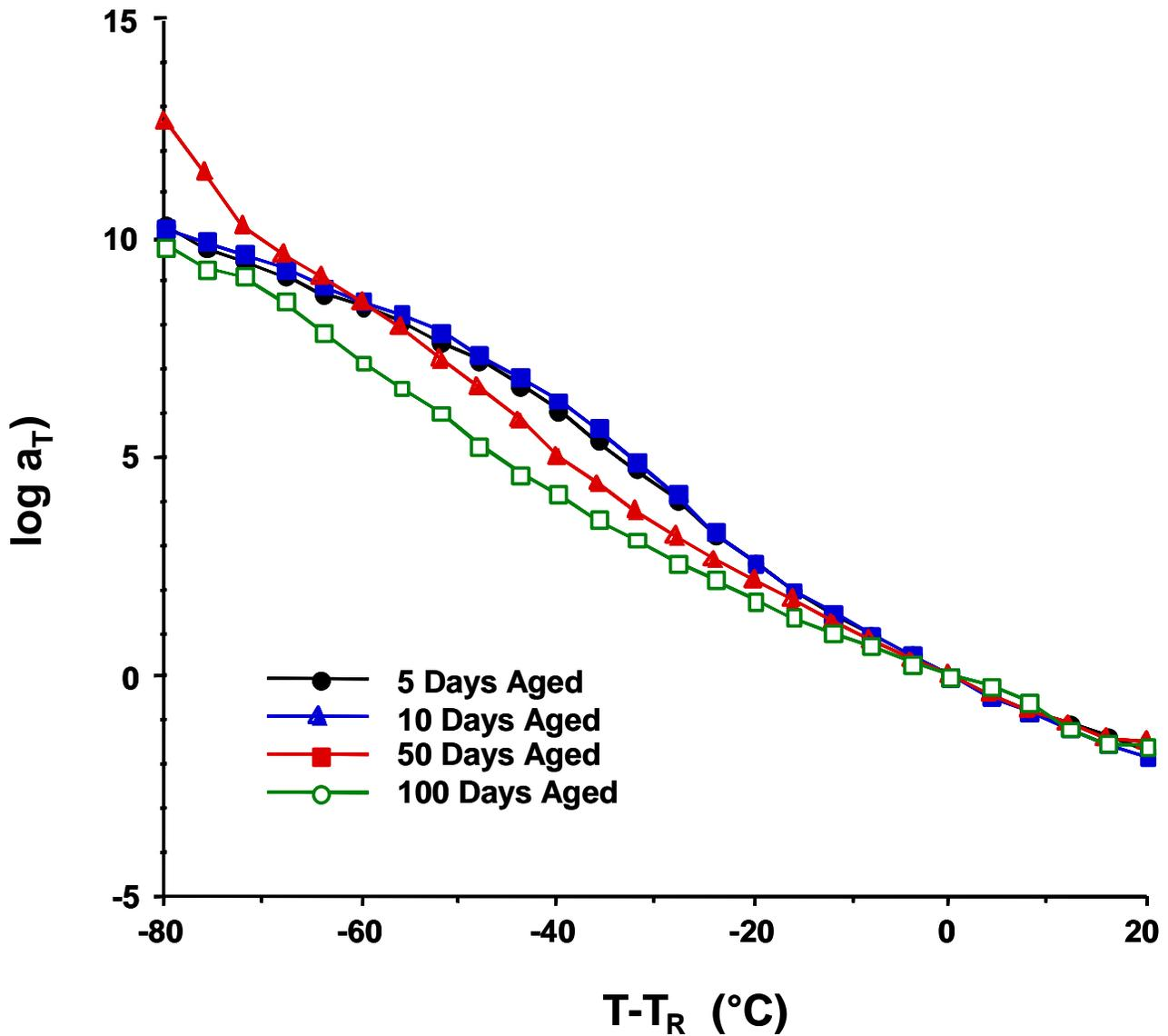
**Figure 4-33.** Shift factor plots for neat cyanate ester resins aged in an air atmosphere at 177°C for times shown. These plots correspond to the master curves displayed in Figure 4-30 and Figure 4-31.
