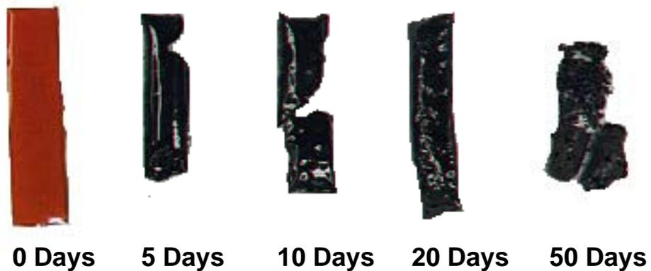
**Figure 4-46.** Visual Examination of neat cyanate ester resins aged at 260°C. Photographs of actual samples are displayed
