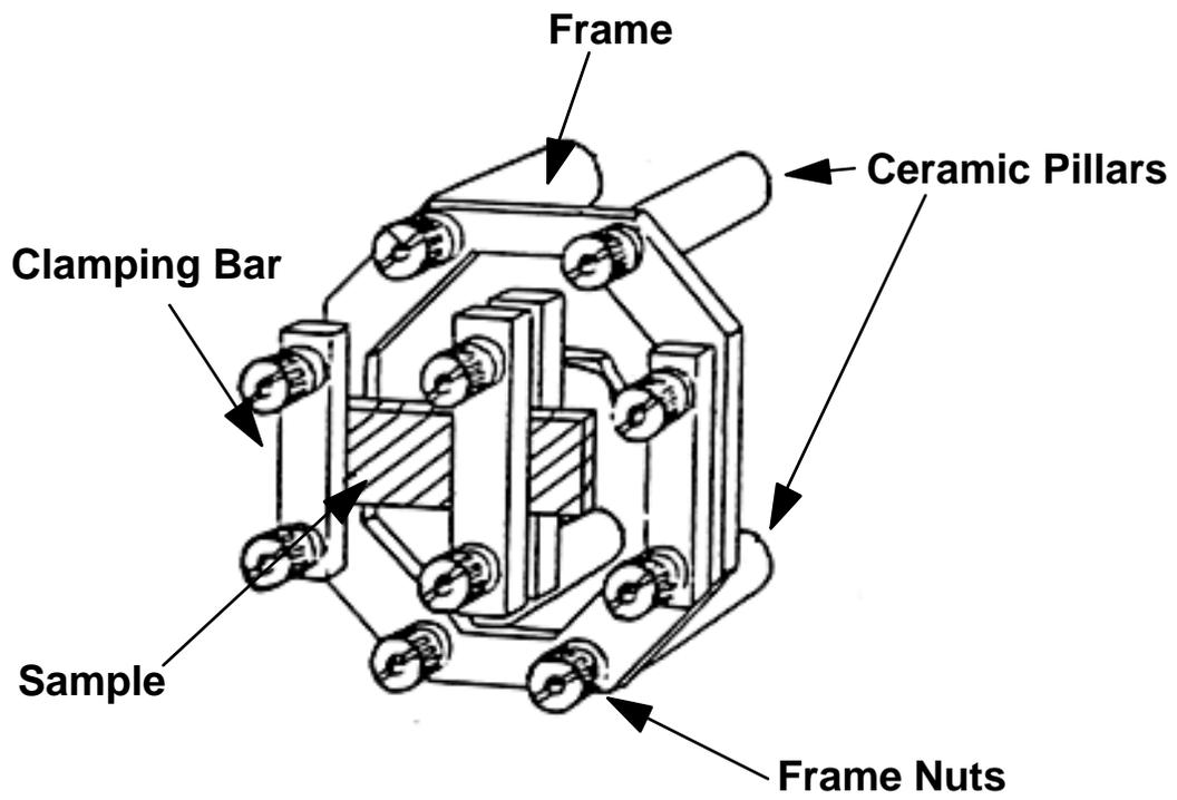
**Figure 3-2.** Schematic representation of single cantilever bending mode DMTA
