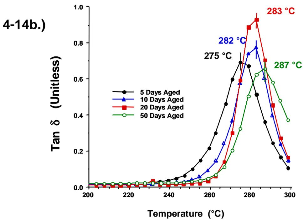
**Figure 4-14.** Mechanical data displayed as a function of temperature for neat cyanate ester resins aged in nitrogen at 260 $^{\circ}\text{C}$ .
