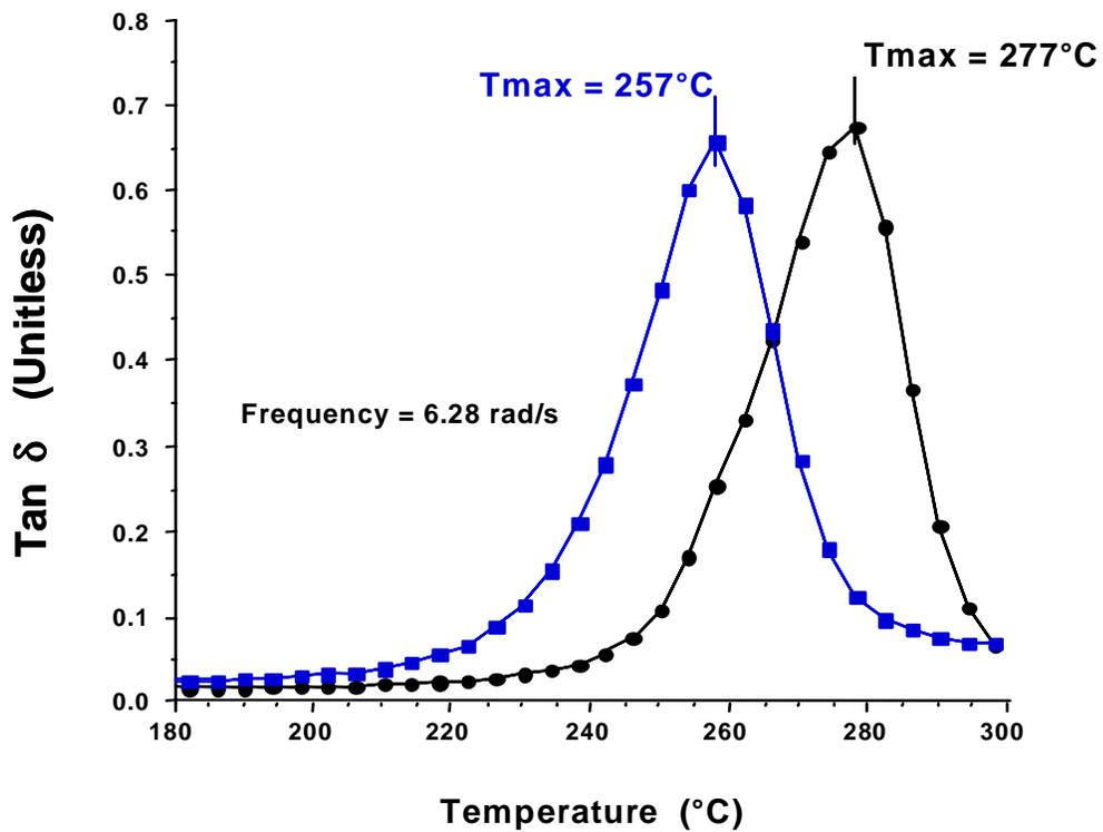
**Figure 4-9.** Mechanical data displayed as a function of temperature for the quenched and annealed samples. Samples were prepared in an air atmosphere; mechanical testing was performed under nitrogen.
