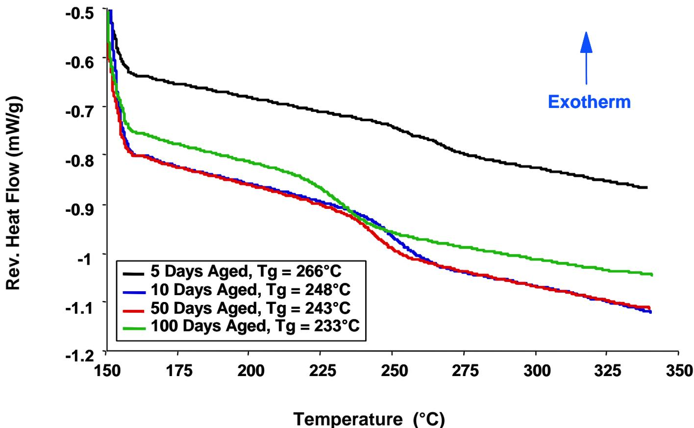
**Figure 4-40.** Modulated DSC scans of 25% thermoplastic toughened cyanate ester resin samples aged in an air atmosphere at 177°C for the times shown. Cure schedule was one hour at 150°C and two hours at 250°C as a post-cure. T<sub>g</sub> was determined using the TA Universal Analysis Software. The midpoint of change in the reversible heat flow was used as the measured value.
