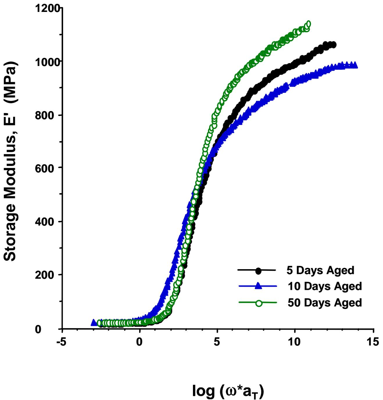
**Figure 4-18.** Storage modulus master curves for cyanate ester resin aged in a nitrogen atmosphere at 177°C for times shown.
