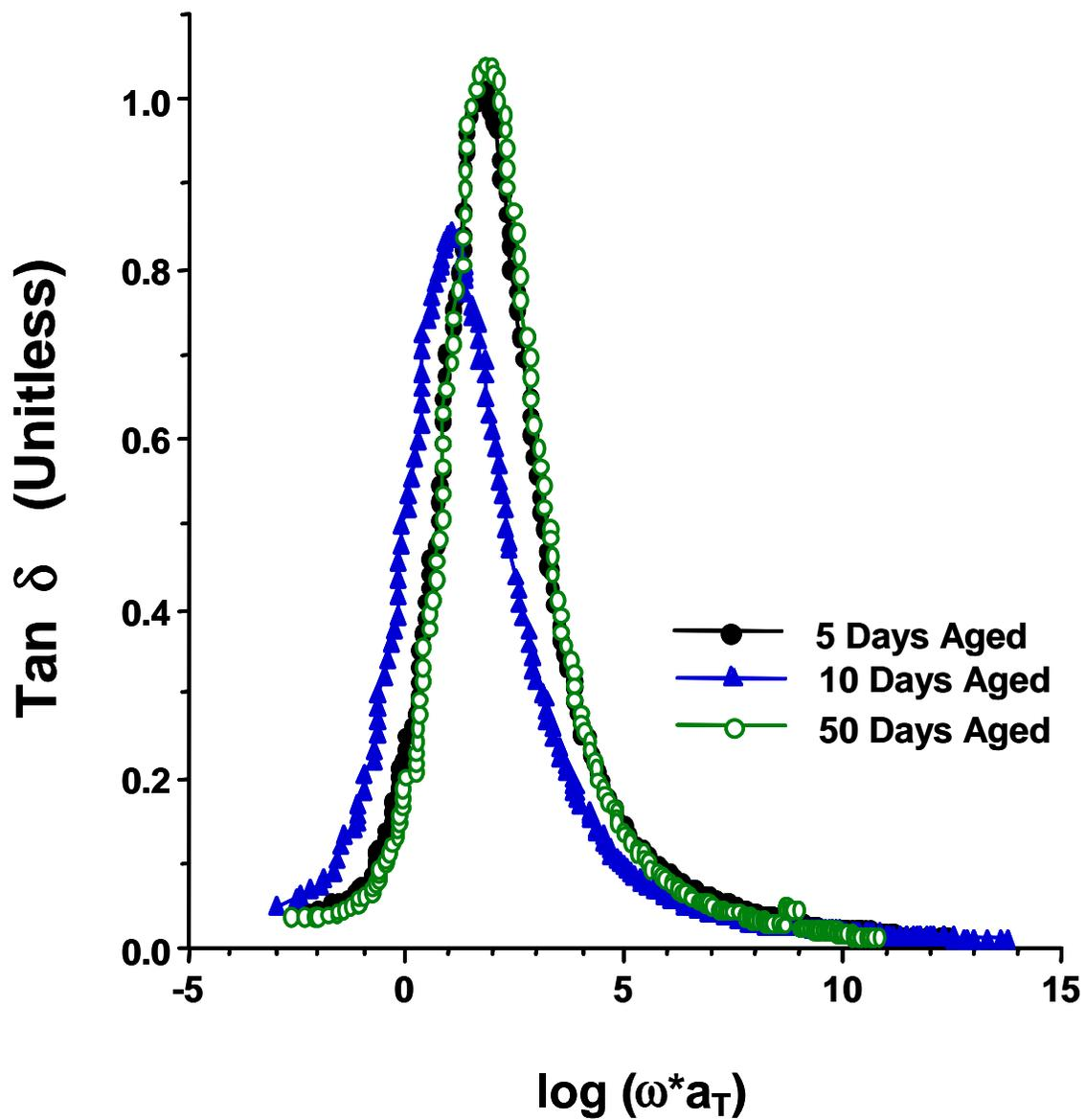
**Figure 4-19.** Tangent  $\delta$  master curves for cyanate ester resins aged in a nitrogen atmosphere at 177°C for times shown.
