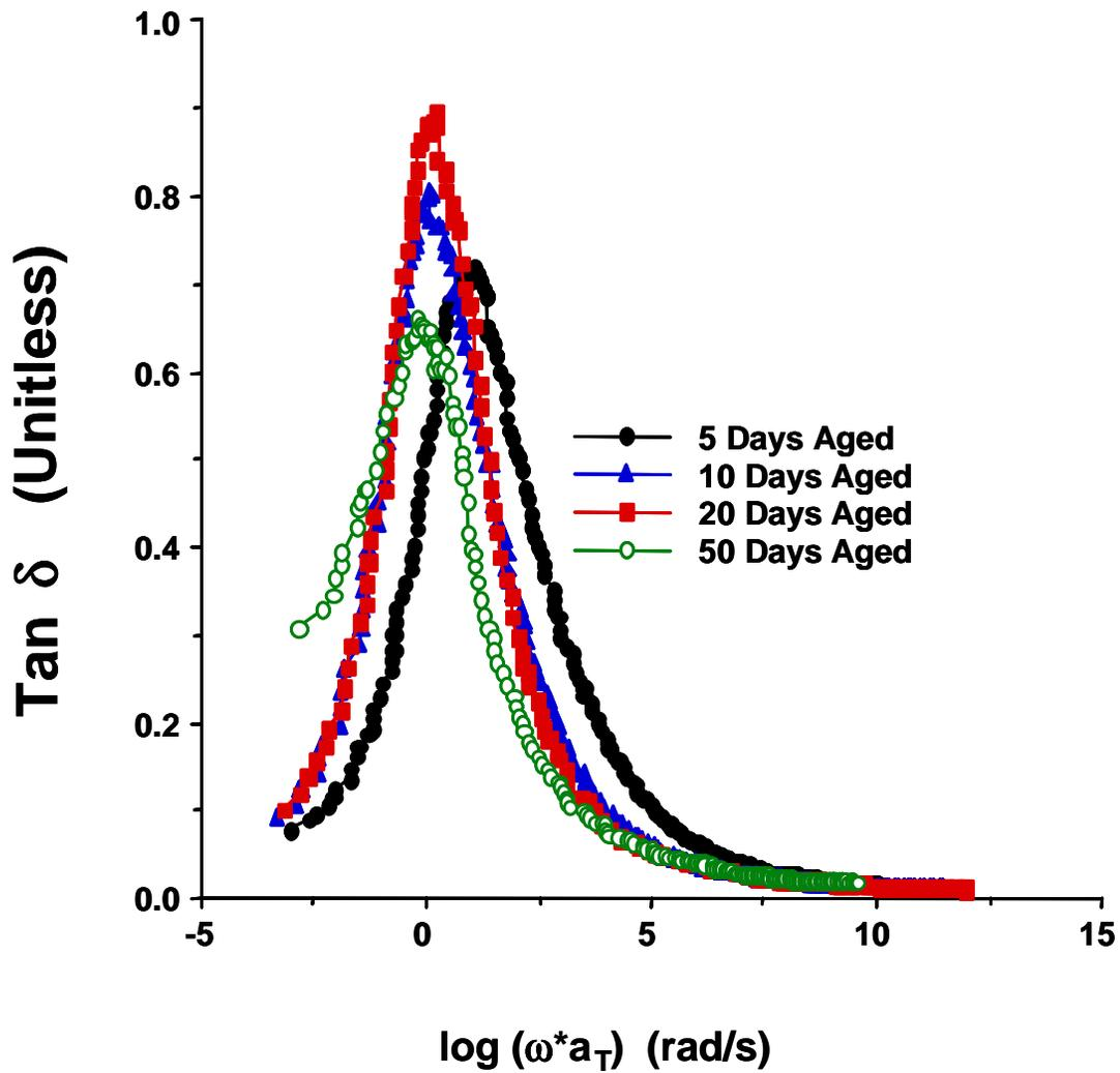
**Figure 4-12.** Bending  $\tan \delta$  master curves of neat cyanate ester resins. A comparison of samples aged in nitrogen at 260°C for varying amounts of time.
