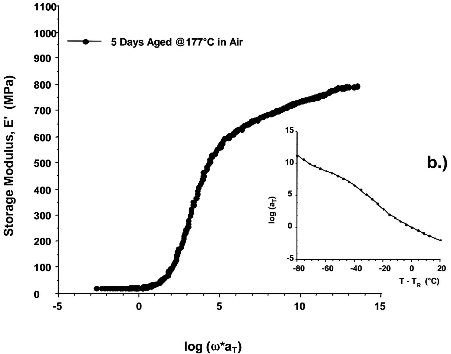
**Figure 4-2.** Master curve produced from time-temperature superpositioning.
