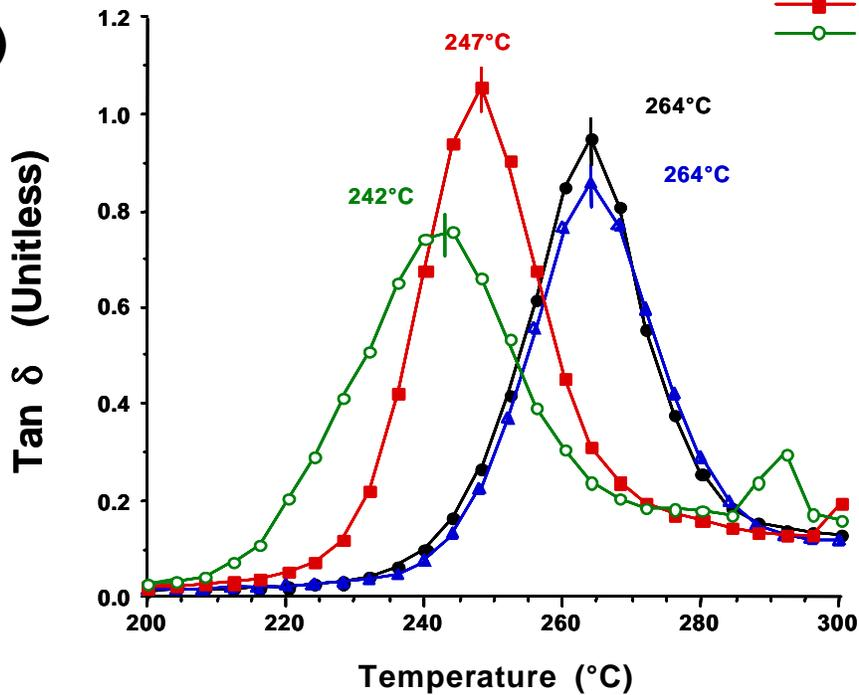
**Figure 4-39.** Rearranged data for 25% thermoplastic toughened cyanate ester resins aged in an air atmosphere at 177 $^{\circ}\text{C}$  for times shown. Data at a frequency of 1 Hz is represented for examination on the temperature axis.
