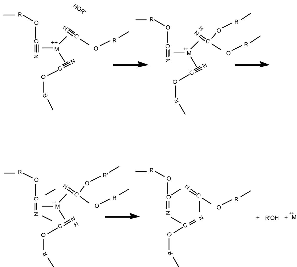
Scheme 3-2. Trimerization Catalyzed by Transition Metal Carboxylates and Active Hydrogens (nonyl phenol)
