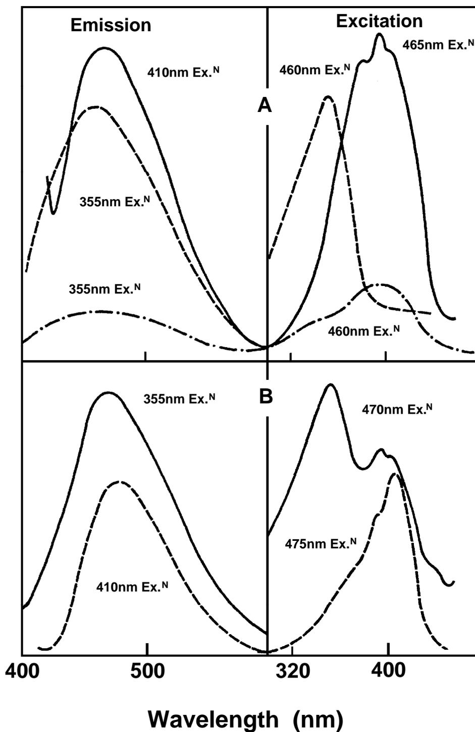
**Figure 2-7.** Luminescence emission from aramid films at 77K: poly(m-phenylene 1,3-phthalamide). (157)
