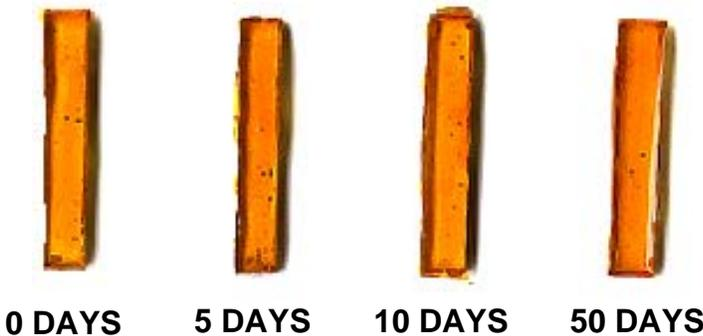
**Figure 4-29.** Visual examination of neat cyanate ester resins after aging at 177°C for the displayed time in the corresponding atmosphere
