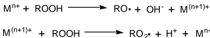
**Scheme 2-13** Acceleration of Thermal Oxidative Polymer Degradation by Transition Metals
