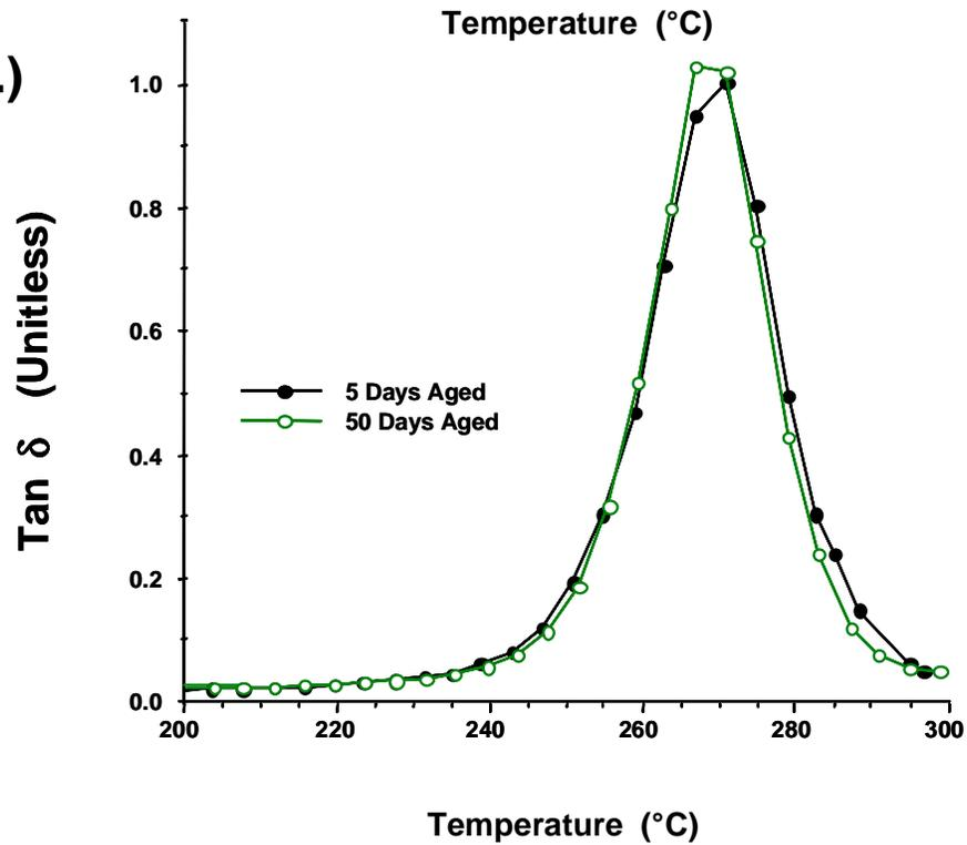
**Figure 4-24.** Continuous sweep thermal scans of 5 and 50 day aged samples at a frequency of 1 Hz.
