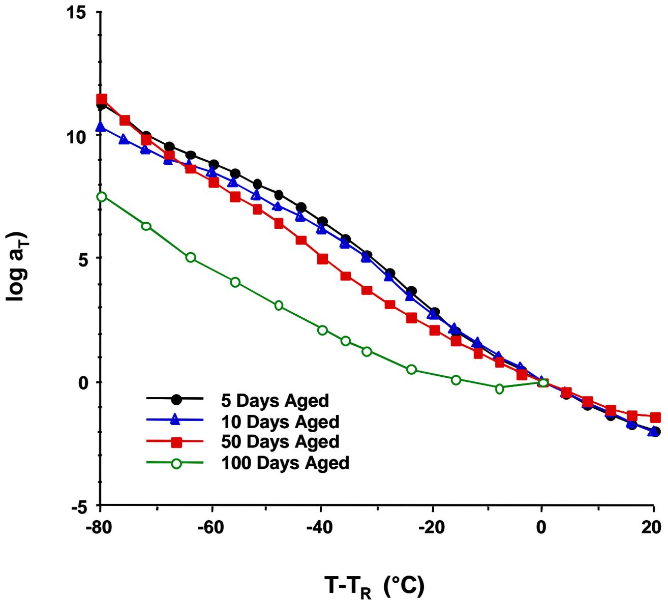
**Figure 4-27.** Shift factor plots for neat cyanate ester resins aged in an air atmosphere at 177°C for times shown. These plots correspond to the master curves displayed in Figure 4-25 and Figure 4-26.
