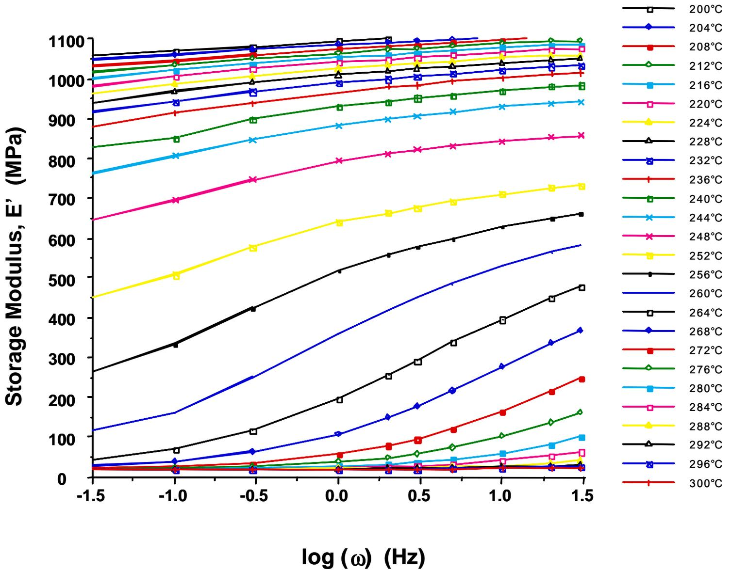
**Figure 4-1.** Set of isothermal curves developed by DMA in step-isothermal mode. Data collected from unmodified Cyanate ester resin aged for five days in an air atmosphere
