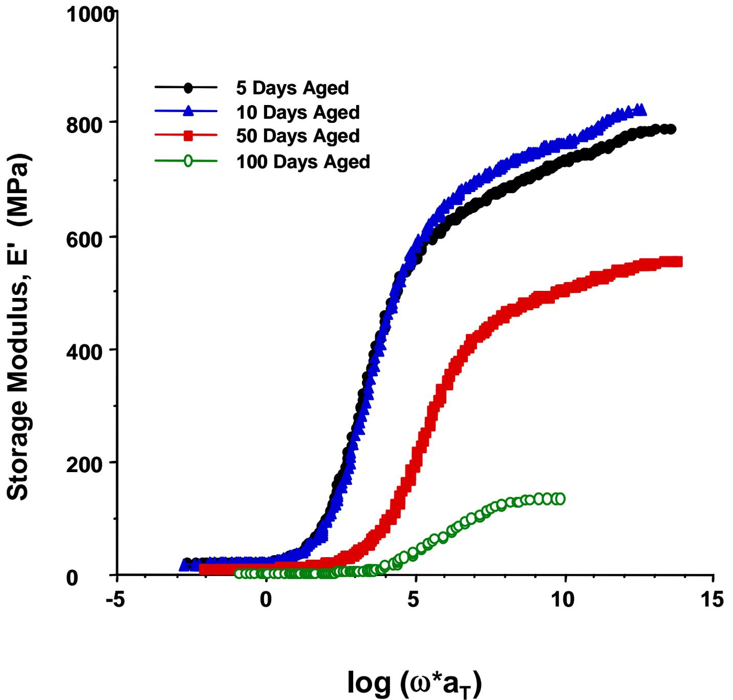
**Figure 4-4.** Family of master curves developed for neat cyanate ester resins at 177°C. The samples were aged in an air atmosphere for the times shown.
