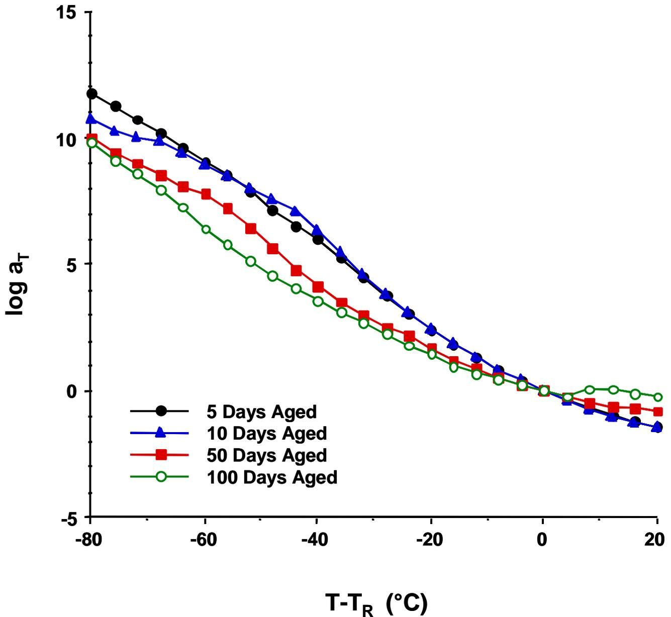
**Figure 4-38.** Shift factor plots for 25% thermoplastic toughened cyanate ester resins aged in an air atmosphere at 177°C for times shown. Plot corresponds to master curves displayed in Figure 4-36 and Figure 4-37.
