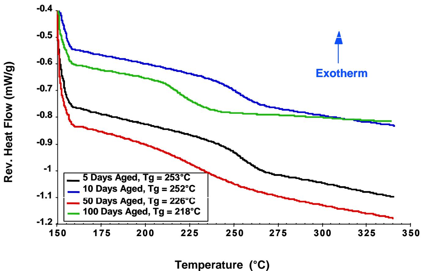
**Figure 4-35.** Modulated DSC scans of neat cyanate ester resin samples aged in an air atmosphere at 177°C for the times shown. Cure schedule was three hours at 250°C. T<sub>g</sub> was determined using the TA Universal Analysis Software. The midpoint of change in the reversible heat flow was used as the measured value.
