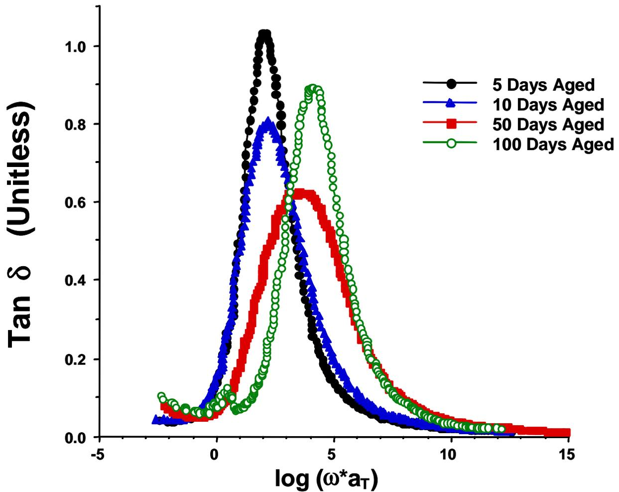
**Figure 4-32.** Tangent  $\delta$  master curves for neat cyanate ester resins aged in an air atmosphere at 177°C for times shown. Cure schedule was three hours at 250°C.
