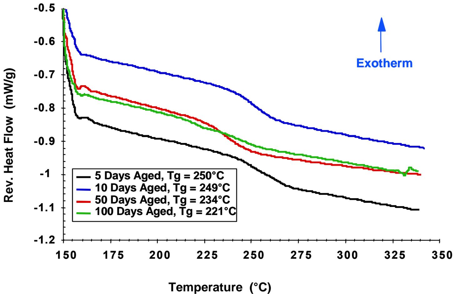
**Figure 4-45.** Modulated DSC scans of 25% thermoplastic toughened cyanate ester resin samples aged in an air atmosphere at 177°C for the times shown. Cure schedule was three hours at 250°C. T<sub>g</sub> was determined using the TA Universal Analysis Software. The midpoint of change in the reversible heat flow was used as the measured value.
