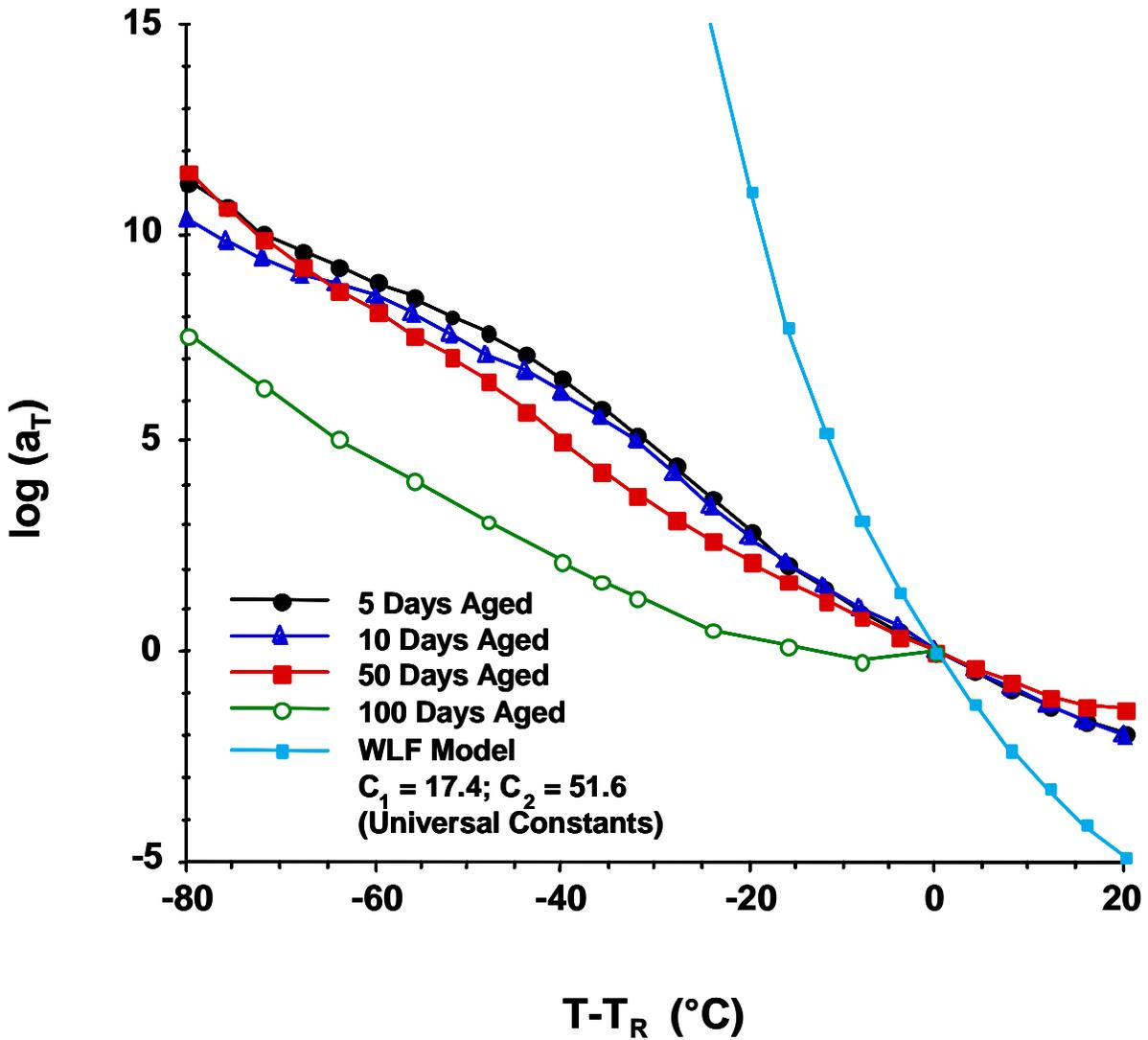
**Figure 4-5.** Shift factor plot data against reduced temperature. Data corresponds to master curves in Figure 4-4. WLF model calculated using universal constants.
