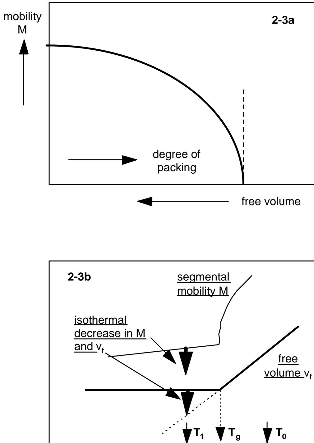
**Figure 2-3.** Illustration of the free-volume concept and its application to the aging problem.(70)
