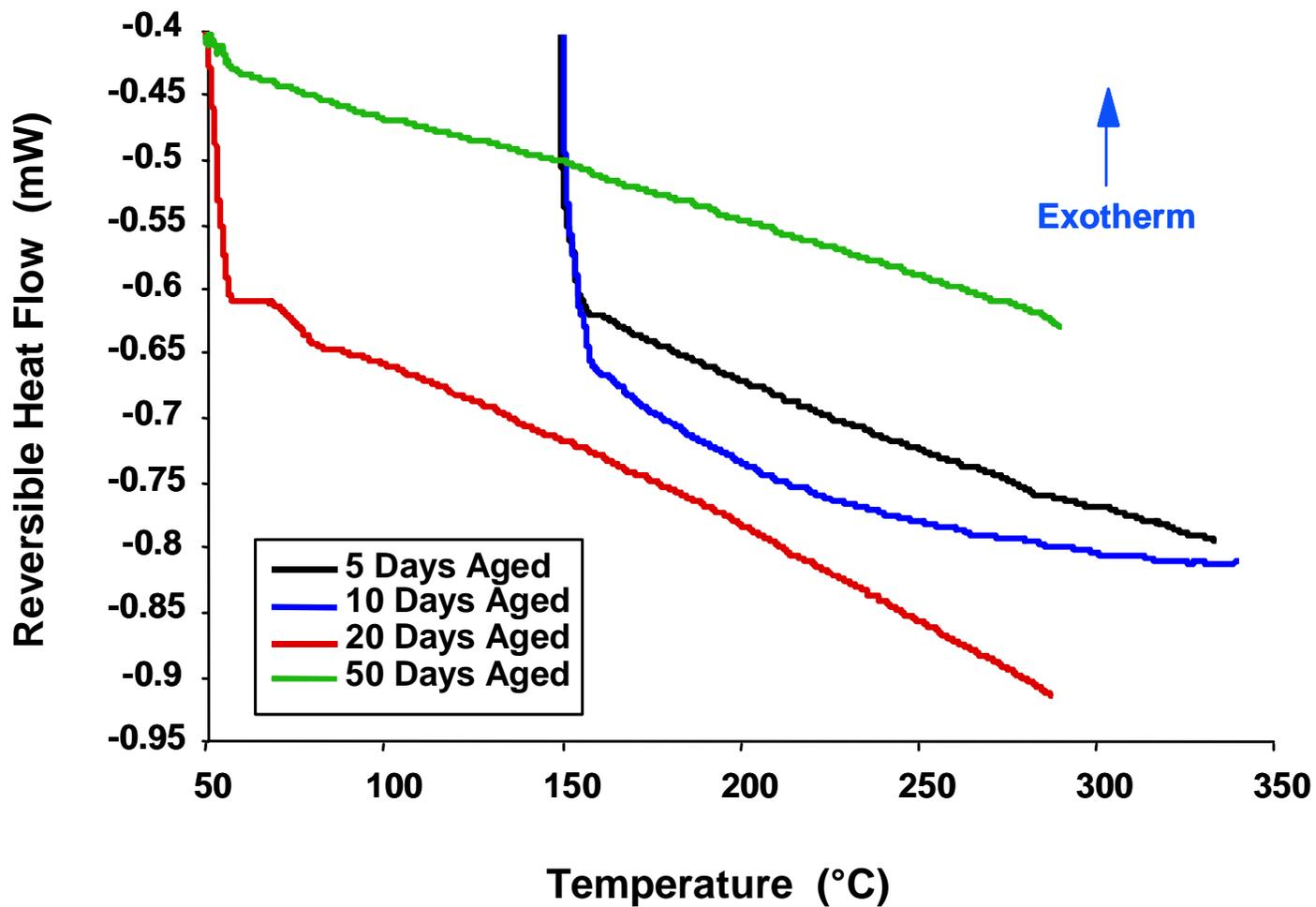
**Figure 4-47.** Modulated DSC scans of neat cyanate ester resin samples aged in an air atmosphere at 260°C for the times shown. No discernable  $T_g$  observed.
