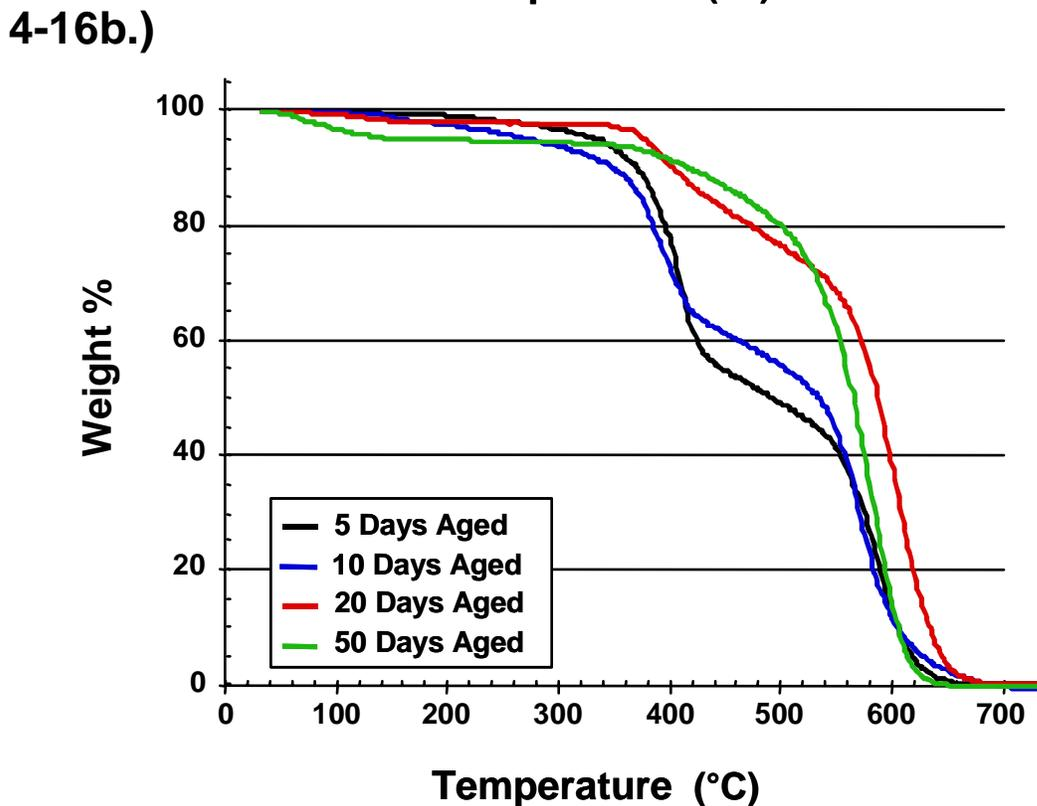
**Figure 4-16.** TGA comparison of neat cyanate ester resins aged at 260°C. Thermal sweeps performed in Air at 10°C/min.
