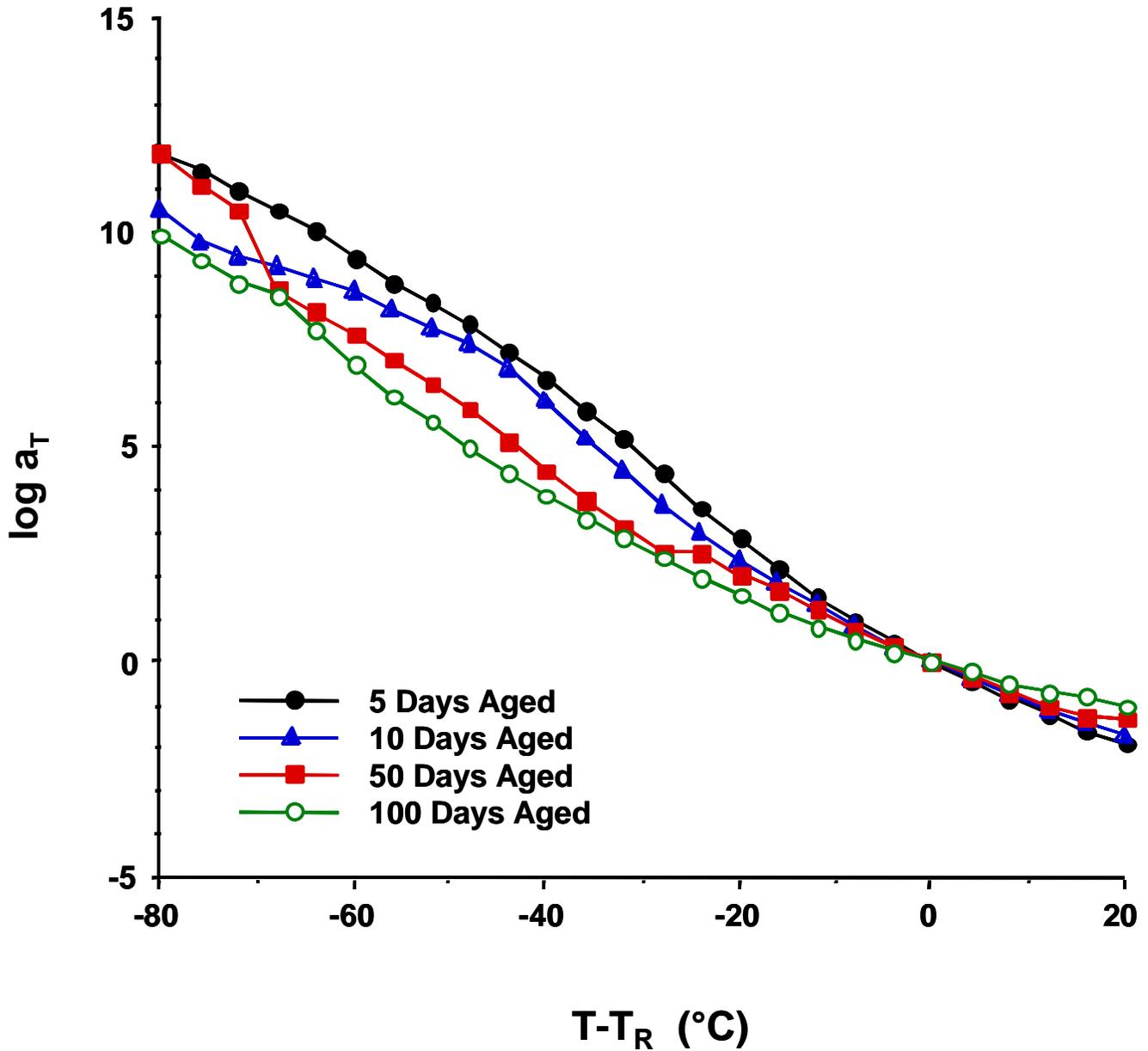
**Figure 4-43.** Shift factor plots for 25% thermoplastic toughened cyanate ester resins aged in an air atmosphere at 177°C for times shown. Plot corresponds to master curves displayed in Figure 4-41 and Figure 4-42.
