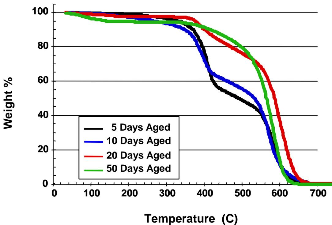
**Figure 4-49.** TGA thermal traces in air of neat cyanate ester resins aged at 260°C for times shown.
