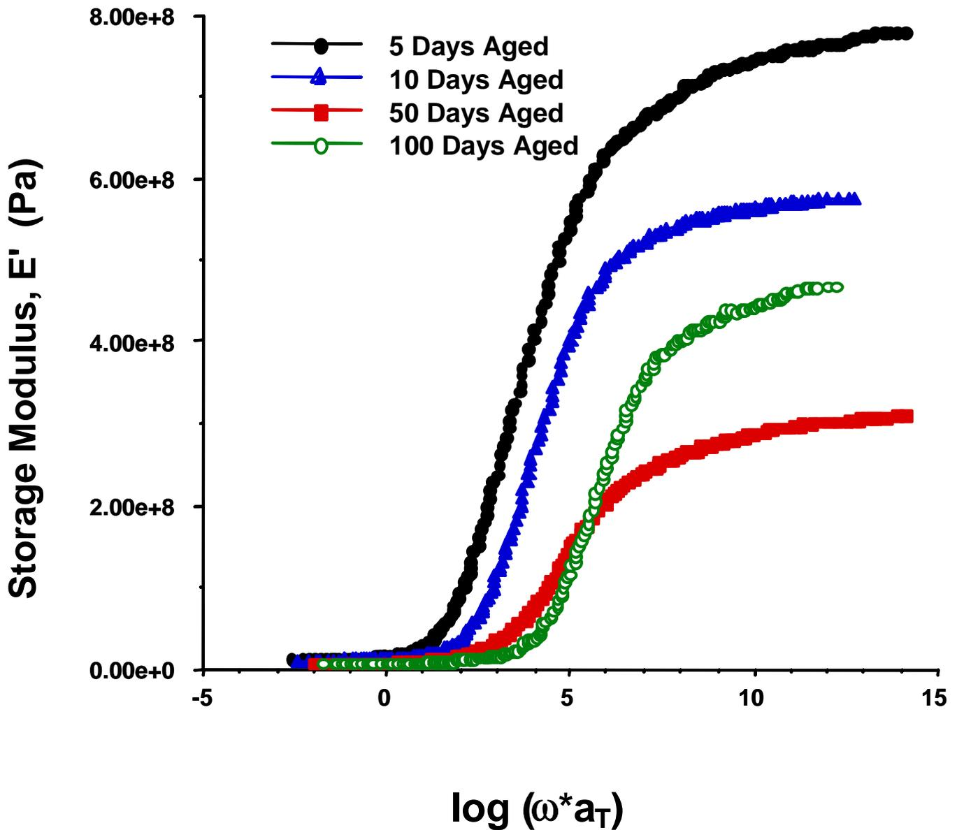
**Figure 4-41.** Storage modulus master curves for 25% thermoplastic toughened cyanate ester resins aged in an air atmosphere at 177°C for times shown. Cure schedule was one hour at 150°C and two hours at 250°C as a post-cure.
