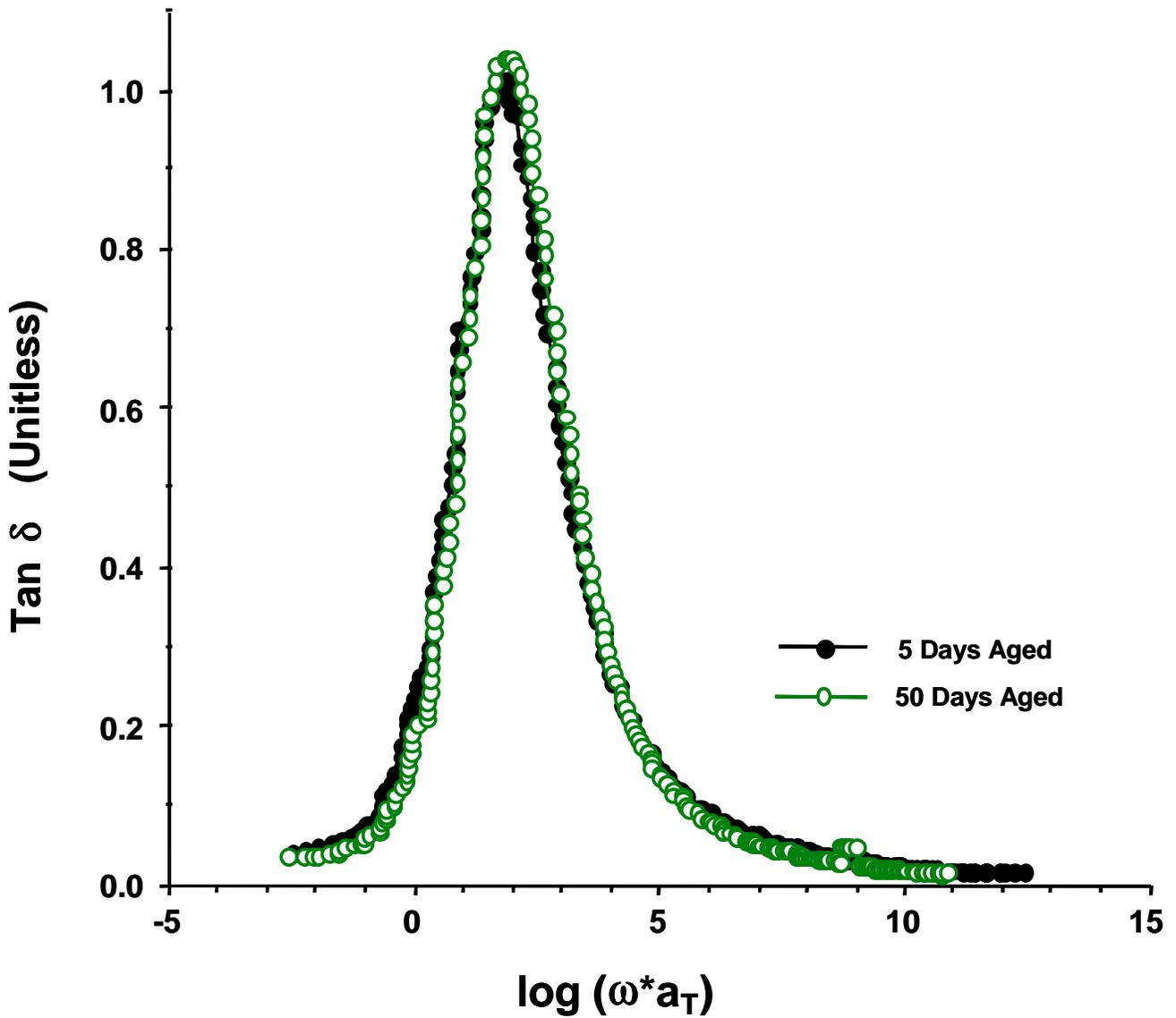
**Figure 4-23.** Tan  $\delta$  master curves (less 10 days aged) for cyanate ester resin aged in a nitrogen atmosphere at 177°C for times shown.
