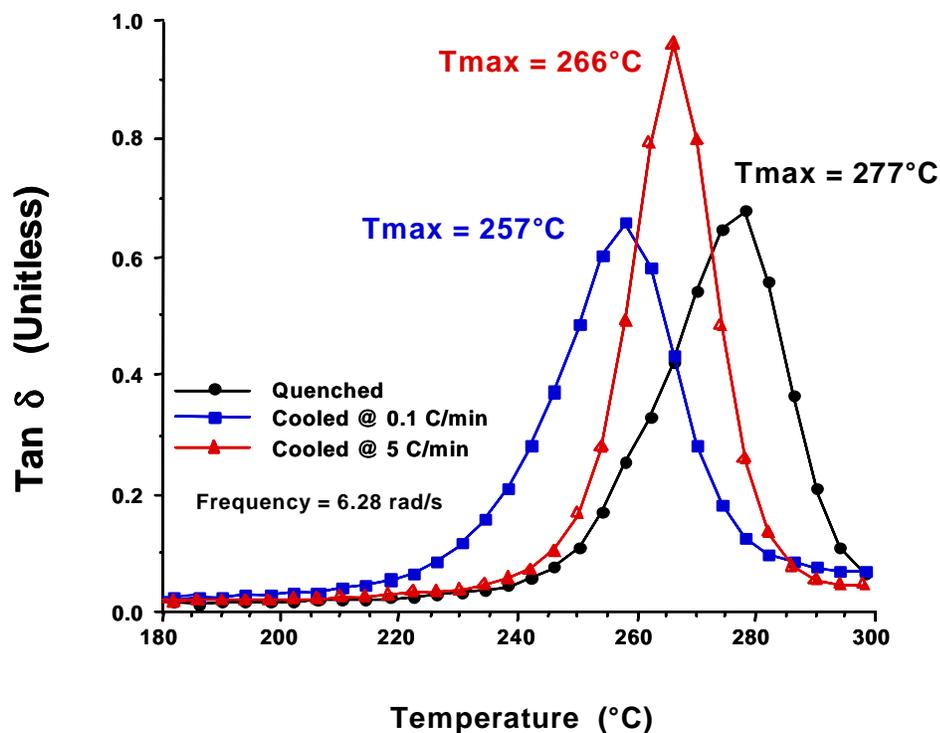
**Figure 4-10.** Mechanical data displayed as a function of temperature for the quenched, intermediate and annealed samples. Samples were prepared in an air atmosphere; mechanical testing was performed under nitrogen.
