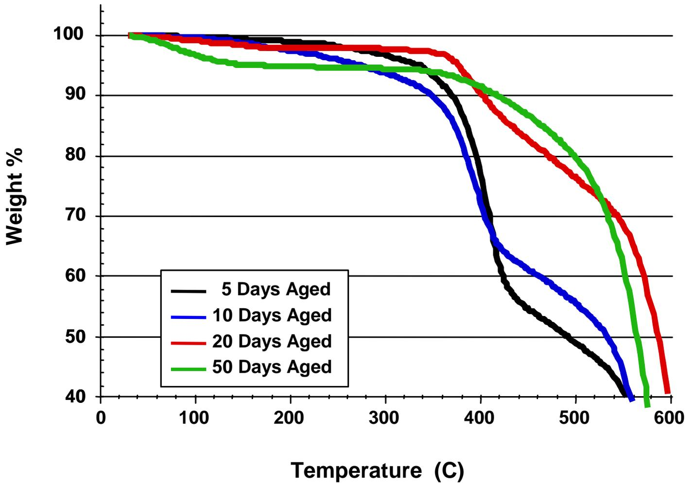
**Figure 4-50.** Expanded view of TGA thermal traces performed in air of neat cyanate ester resin samples aged in air at 260°C for times shown.
