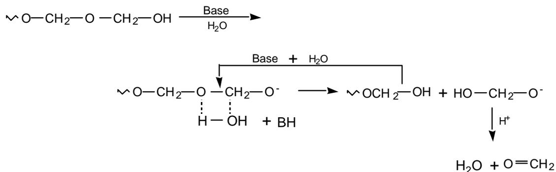
**Scheme 2-12.** Unzipping Process in Polyoxymethylene Under Basic Conditions
