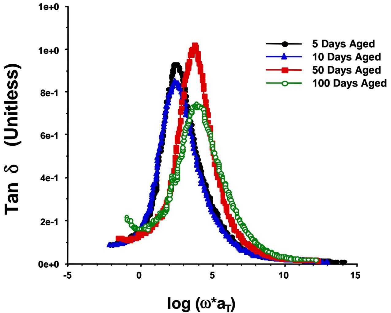
**Figure 4-37.** Tangent  $\delta$  master curves for 25% thermoplastic toughened cyanate ester resins aged in an air atmosphere at 177°C for times shown. Cure schedule was three hours at 250°C.
