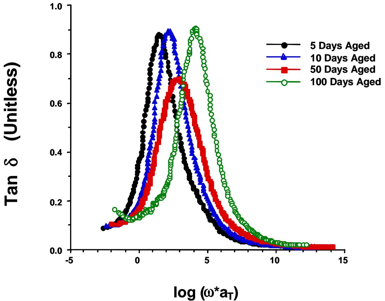
**Figure 4-42.** Tangent  $\delta$  master curves for 25% thermoplastic toughened cyanate ester resins aged in an air atmosphere at 177°C for times shown. Cure schedule was one hour at 150°C and two hours at 250°C as a post-cure.
