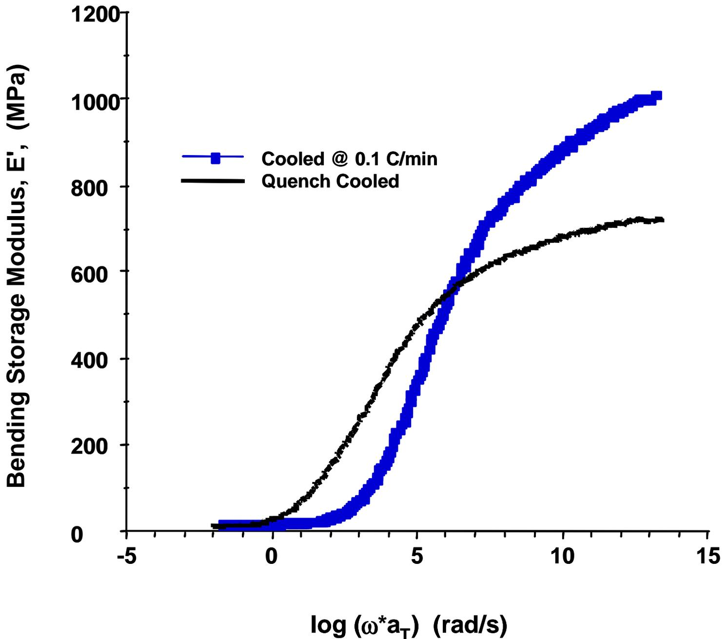
**Figure 4-6.** Bending storage modulus master curves of neat cyanate ester resins. A comparison is made of quench cooled versus annealed (slow cooled) samples. Samples were prepared in an air atmosphere; mechanical testing was performed under nitrogen.
