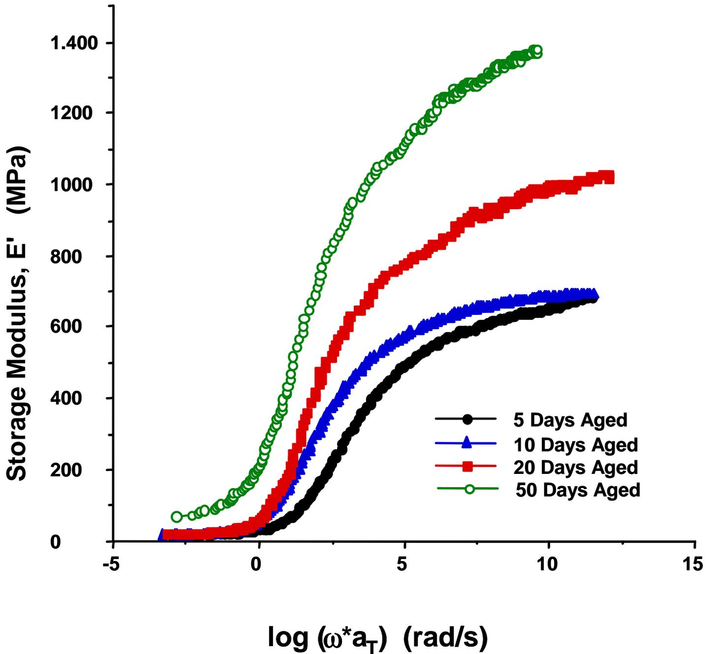
**Figure 4-11.** Bending storage modulus master curves of neat cyanate ester resins. A comparison of samples aged in nitrogen at 260°C for varying amounts of time.
