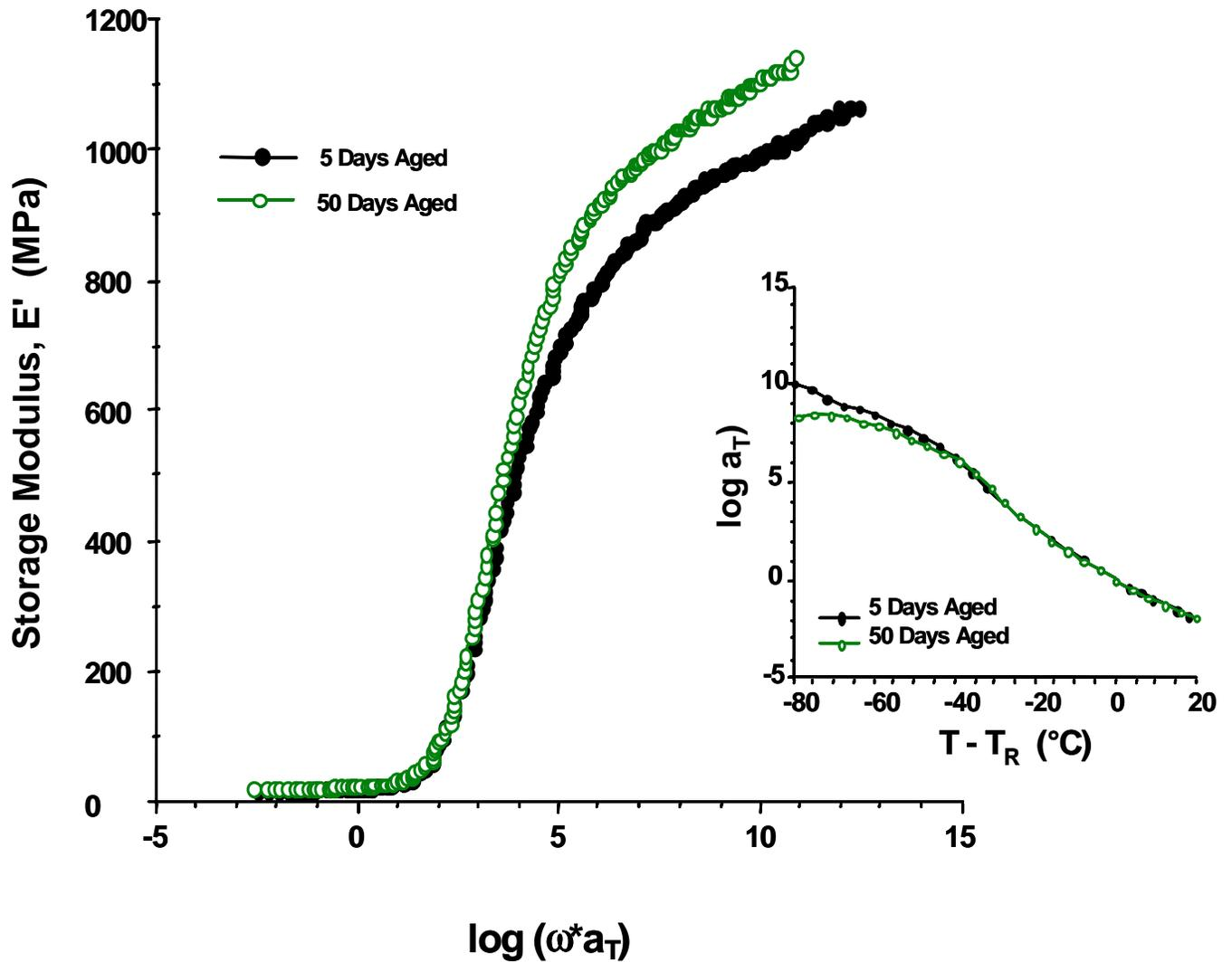
**Figure 4-22.** Storage modulus master curves and shift factor plots (less 10 days aged) for cyanate ester resin aged in a nitrogen atmosphere at 177°C for times shown.
