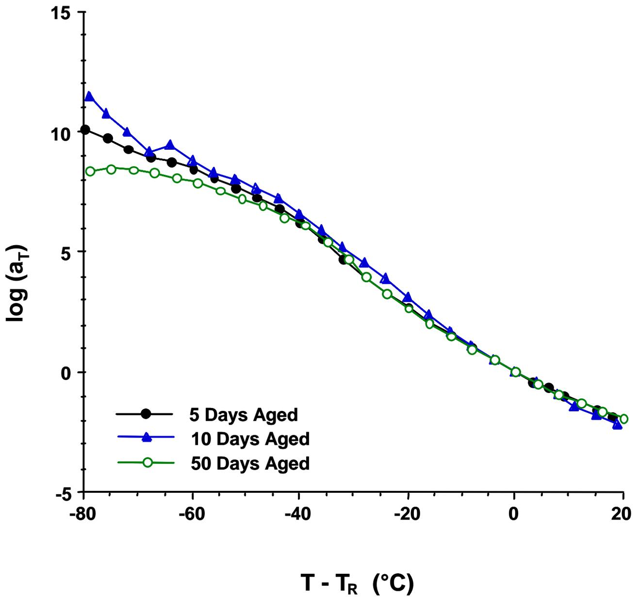
**Figure 4-20.** Shift factor plots for cyanate ester resins aged in a nitrogen atmosphere at 177°C for times shown.
