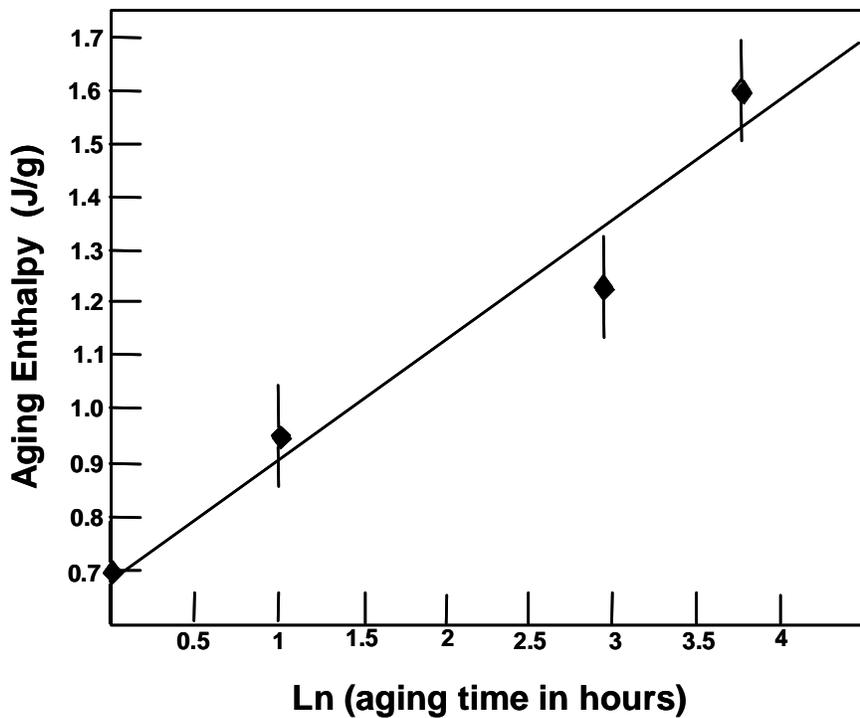
Figure 2-6. a) Changing heat capacity with aging. b) Extent of aging at 12.6 K below  $T_g$ . (102)
