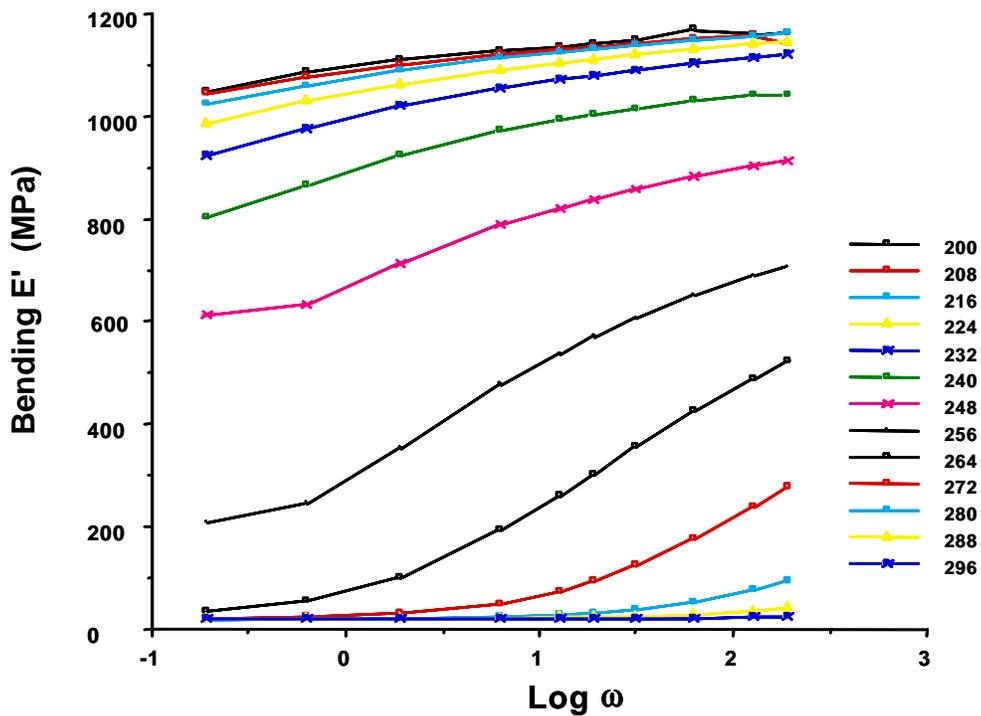
**Figure 3-3.** Typical Raw data collected for master curve development. (5 days aged @  $177^{\circ}\text{C}$  in Air)
