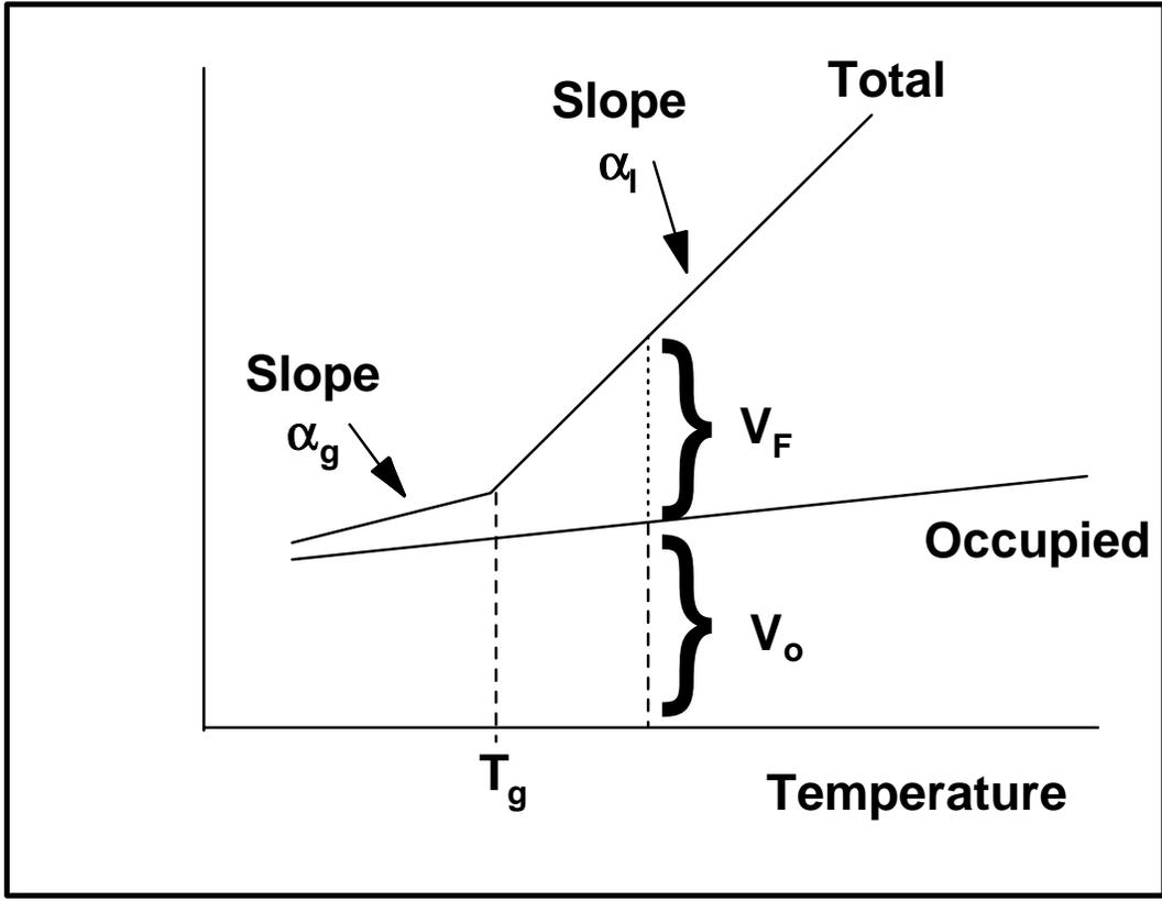
**Figure 2-2.** Total and occupied volumes of a glass forming liquid as a function of temperature.(72)
