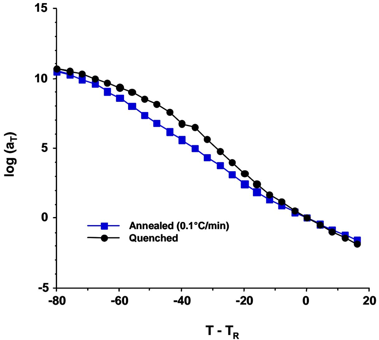
**Figure 4-8.** Shift factor plot generated corresponding to the master curves in Figure 4-6 and Figure 4-7.
