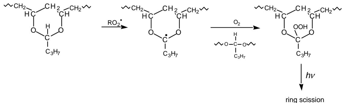
**Scheme 2-10.** Oxidative Ring Scission at Ether Linkages
