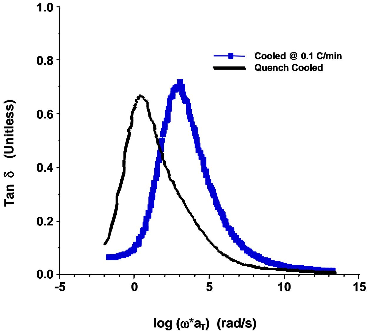
**Figure 4-7.** Bending  $\tan \delta$  master curves of neat cyanate ester resins. A comparison is made of quench cooled versus annealed (slow cooled) samples. Samples were prepared in an air atmosphere; mechanical testing was performed under nitrogen.
