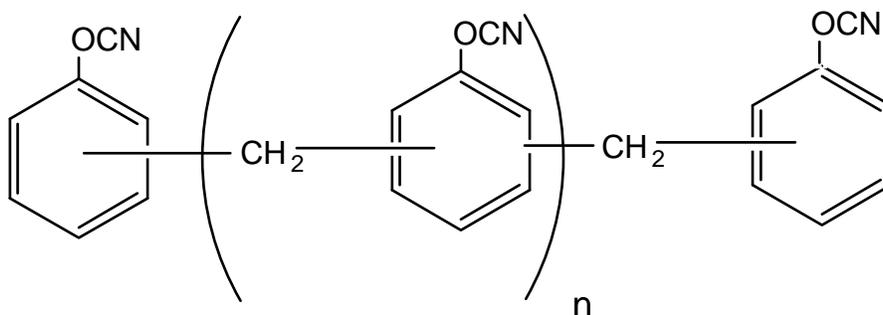
**Scheme 2-6.** General Structure of Phenolic Triazine PT Resins from Allied Signal, Inc.
