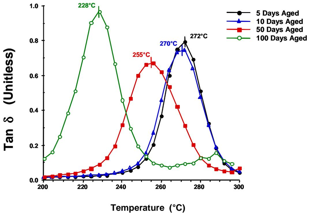
Figure 4-28. Rearranged data at a frequency of 1 Hz for examination on the temperature axis
