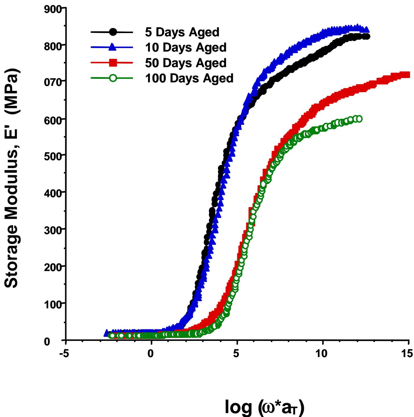
**Figure 4-31.** Storage modulus master curves for neat cyanate ester resin aged in an air atmosphere at 177°C for times shown. Cure schedule was three hours at 250°C.
