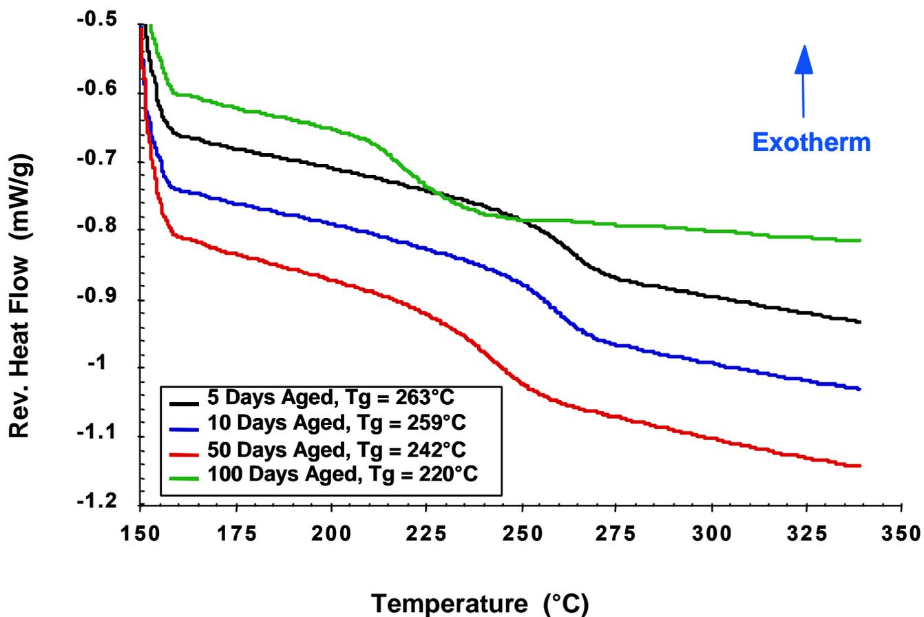
**Figure 4-30.** Modulated DSC scans of neat cyanate ester resin samples aged in an air atmosphere at 177°C for the times shown. Cure schedule was one hour at 150°C and two hours at 250°C as a post-cure. T<sub>g</sub> was determined using the TA Universal Analysis Software. The midpoint of change in the reversible heat flow was used as the measured value.
