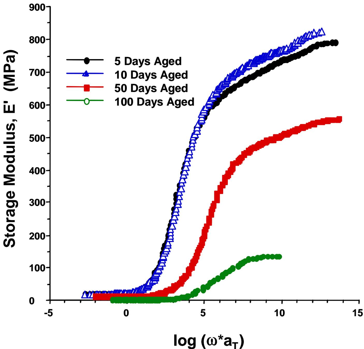
**Figure 4-25.** Storage modulus master curves for neat cyanate ester resin aged in an air atmosphere at 177°C for times shown. Cure schedule was one hour at 150°C and two hours at 250°C as a post-cure.
