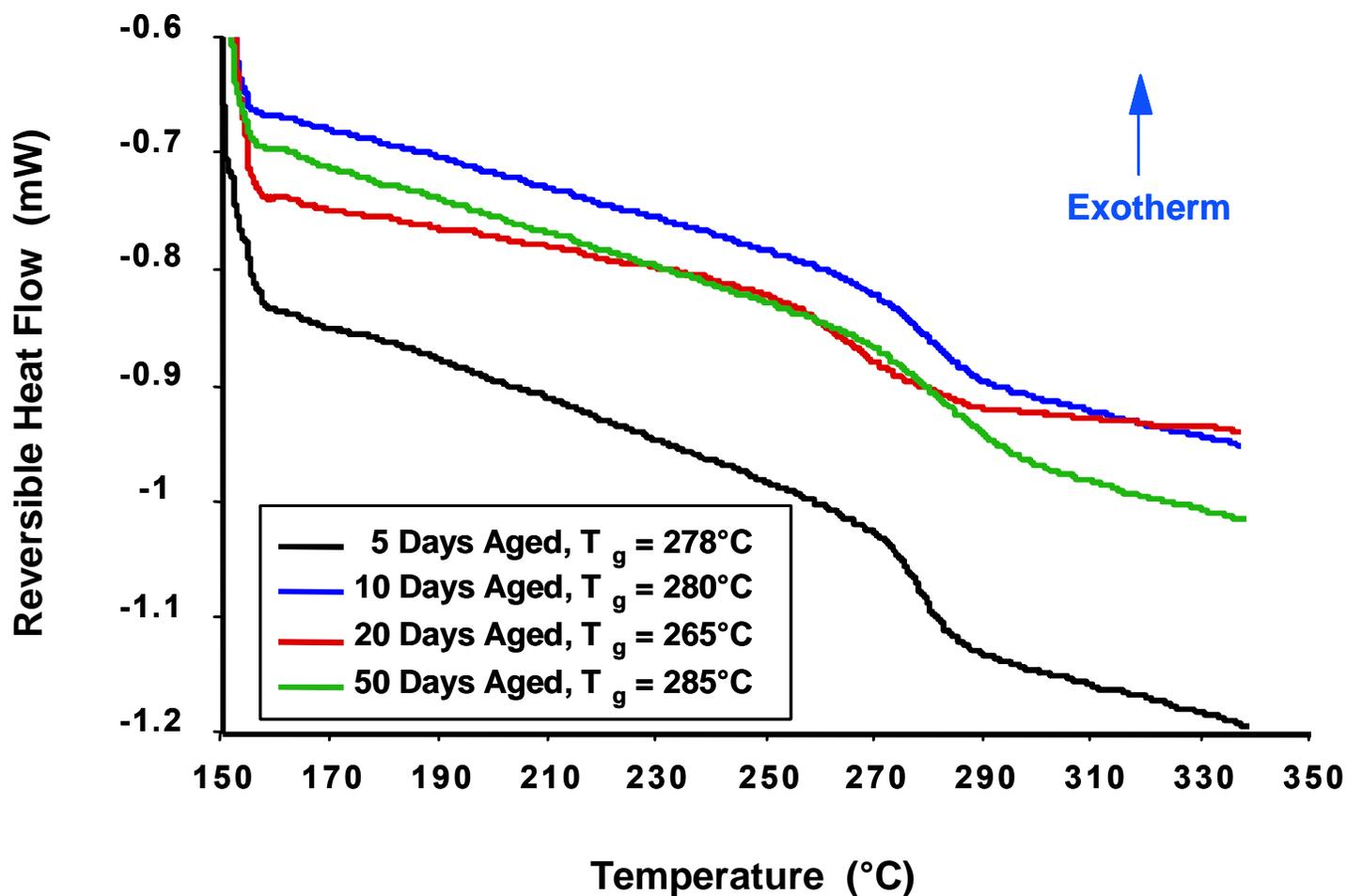
**Figure 4-48.** Modulated DSC scans of neat cyanate ester resin samples aged in a nitrogen atmosphere at 260°C for the times shown. T<sub>g</sub> was determined using the TA Universal Analysis Software. The midpoint of change in the reversible heat flow was used as the measured value.
