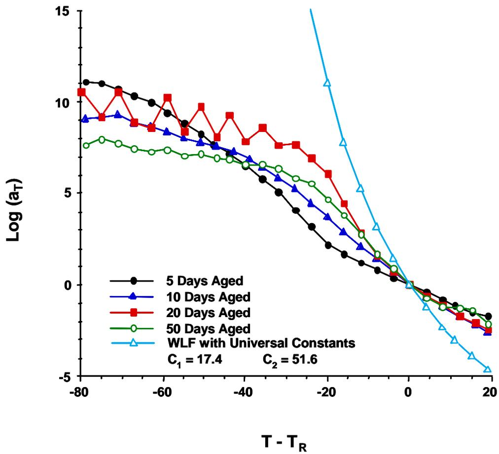
**Figure 4-13.** Shift factor plot generated corresponding to the master curves in Figure 4-11 and Figure 4-12.
