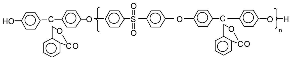
**Scheme 3-3.** Hydroxy Functionalized Poly(arylene ether sulfone)
