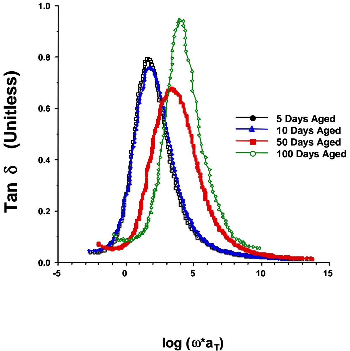
**Figure 4-26.** Tangent  $\delta$  master curves for neat cyanate ester resins aged in an air atmosphere at 177°C for times shown. Cure schedule was one hour at 150°C and two hours at 250°C as a post-cure.
