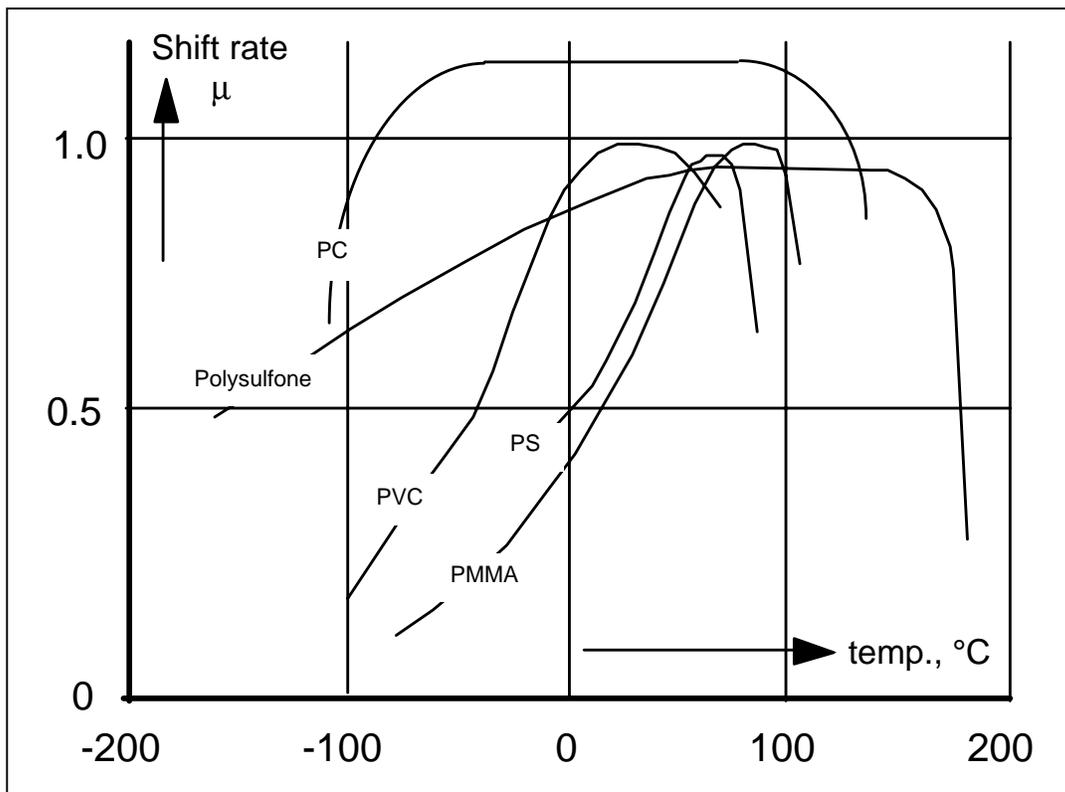
**Figure 2-5.** The shift rate,  $\mu$ , vs. temperature for various polymers. <sup>(70)</sup>
