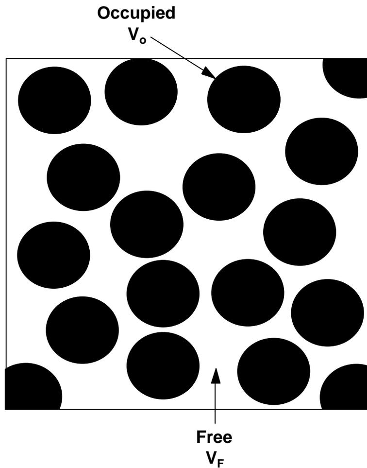
**Figure 2-1.** Simple model of a liquid showing occupied and free volume.(72)
