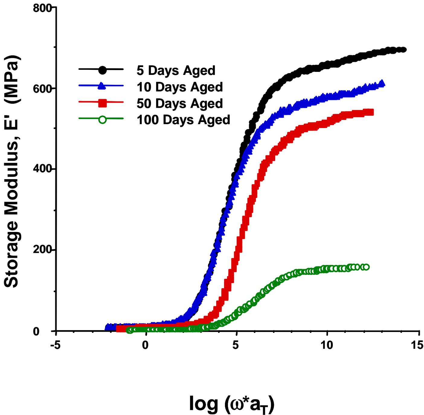
**Figure 4-36.** Storage modulus master curves for 25% thermoplastic toughened cyanate ester resins aged in an air atmosphere at 177°C for times shown. Cure schedule was three hours at 250°C.
