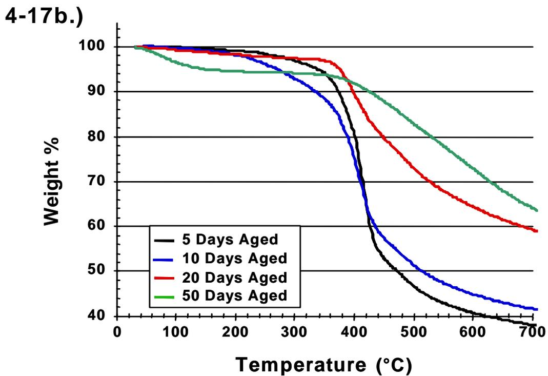
**Figure 4-17.** TGA comparison of neat cyanate ester resins aged at 260°C. Thermal sweeps performed in Nitrogen at 10°C/min.
