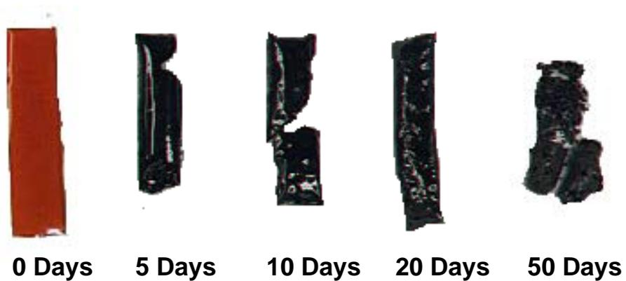
**Figure 4-15.** Visual Examination of neat cyanate ester resins aged at 260°C. Photographs of actual samples are displayed
