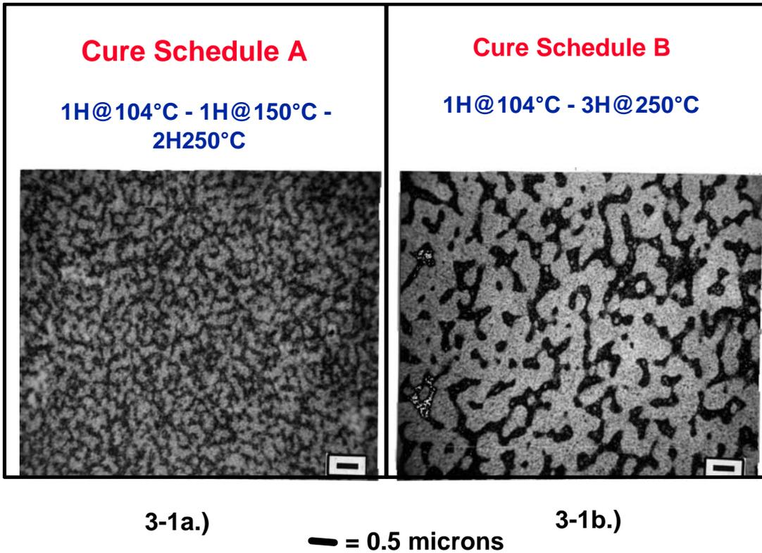
**Figure 3-1.** Scanning electron microscopy (SEM) comparison of two morphologies controlled by cure cycle.
