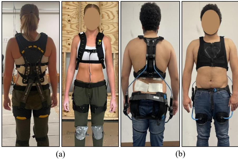
Figure 2. Participants wearing (a) HeroWear Apex (HW) and (b) Laevo Flex (LV) exoskeletons, a demonstration of how both BSEs fit the body on the dorsal and ventral sides.
