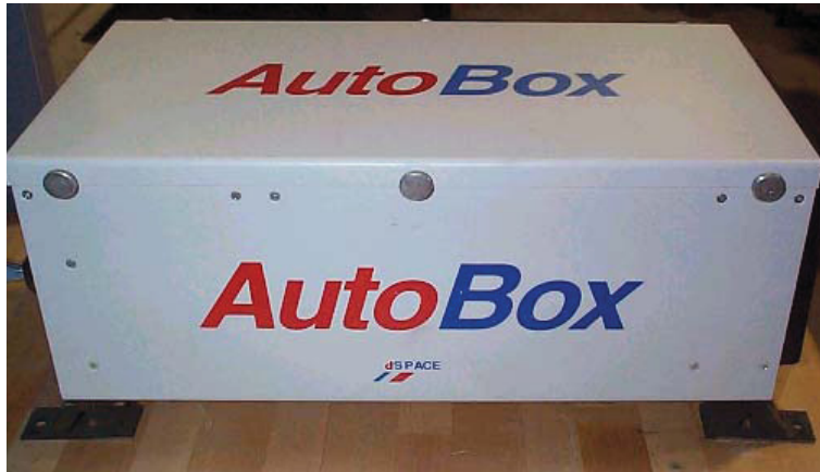
Figure 4-11. dSPACE AutoBox used for digital signal processing
