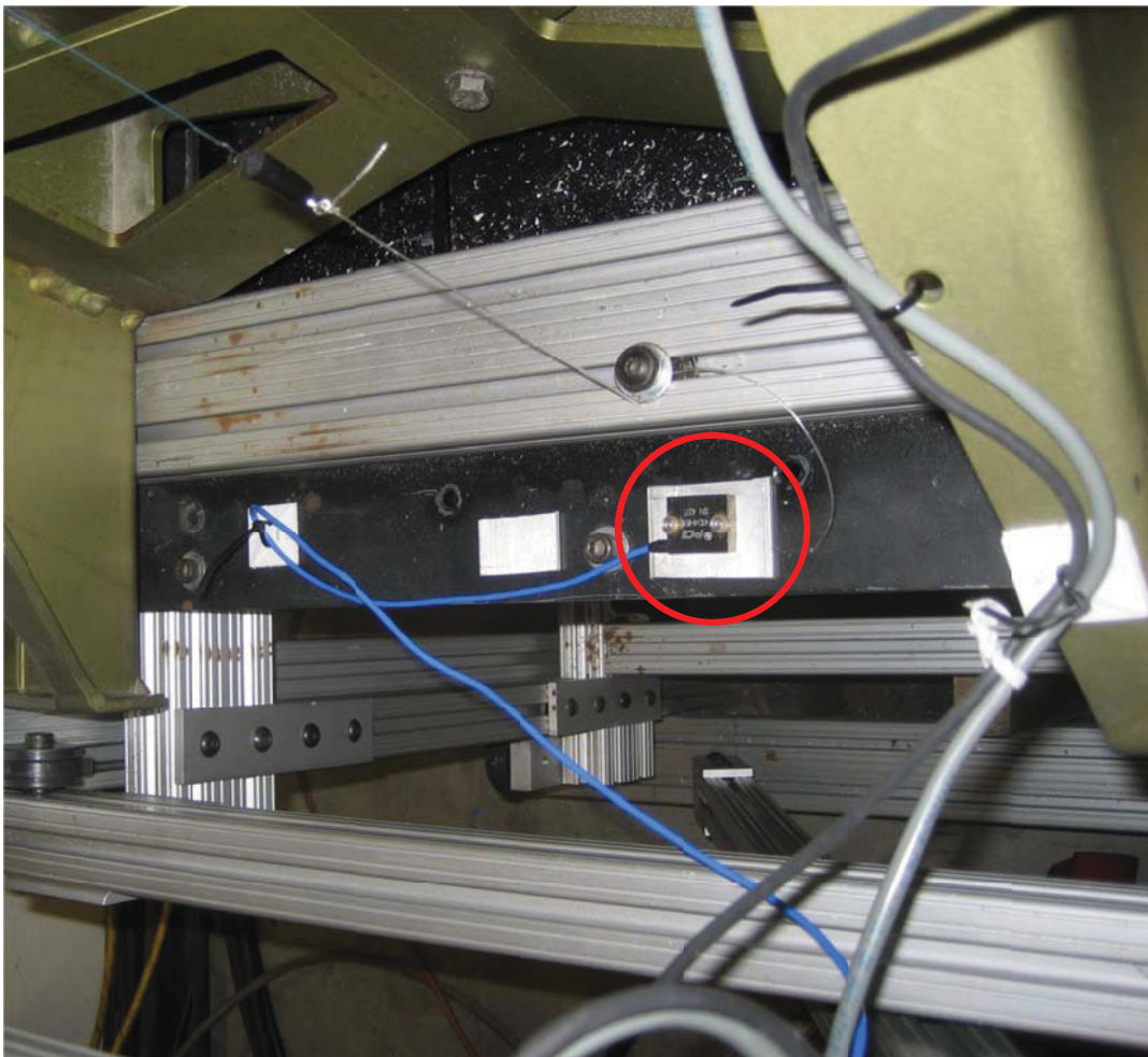
Figure 4-7. MEMS accelerometer, circled in red, mounted on the base of the seat shake rig.
