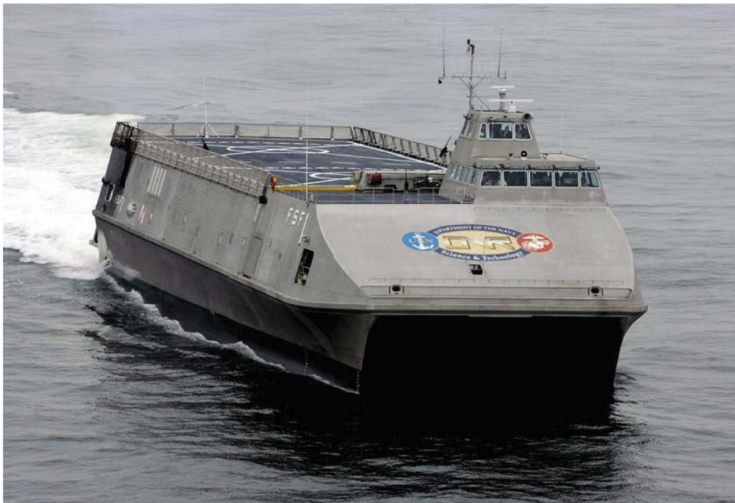
Figure 2-5. Sea Fighter FSF-1 experimental high-speed catamaran used in testing wave slam motion [14].
