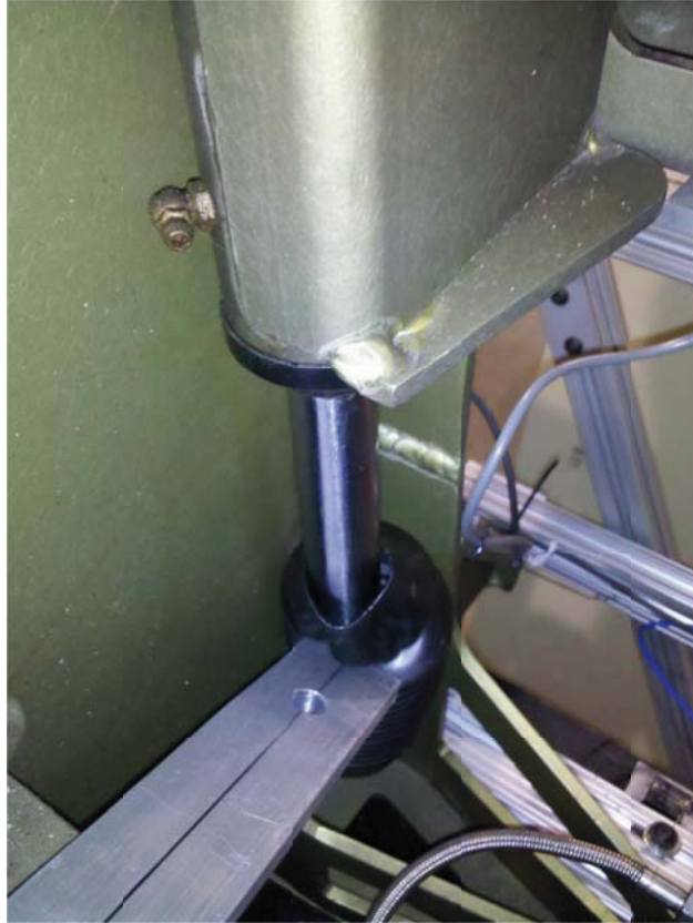
Figure 9-2. Vertical guide assumed to have negligible friction forces present
