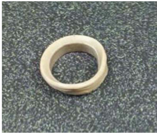
Figure 3-9. Original damaged rod seal removed from the shock assembly.
