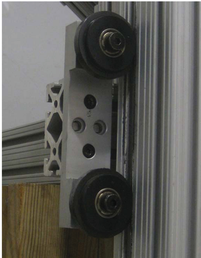
Figure 4-2. Close-up shot of 80/20 rollers used to constrain motion in the horizontal plane while allowing freedom in the vertical.
