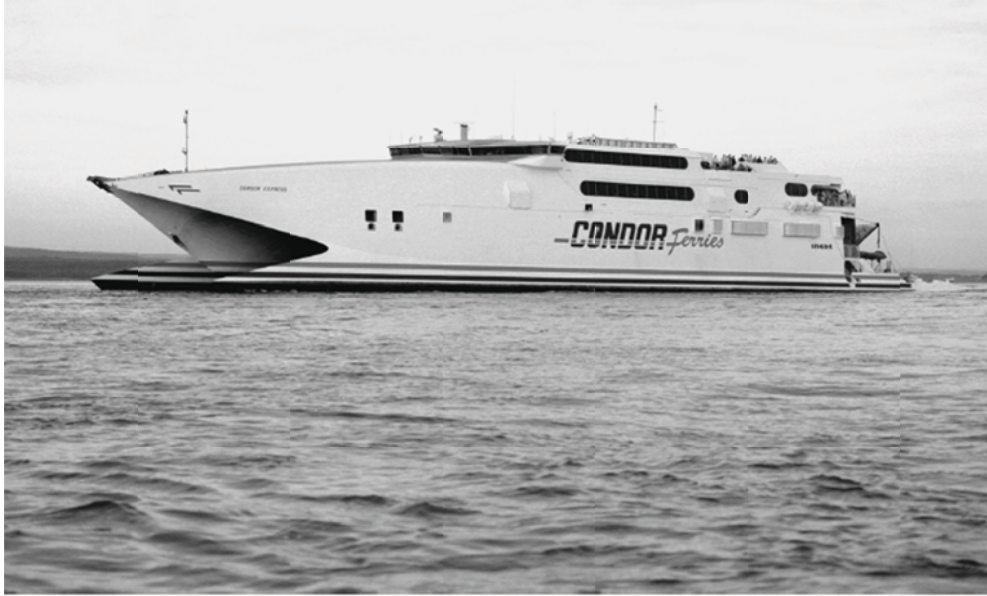
Figure 2-4. High-speed 86 meter Incat ferry used to take wave slamming data while on voyage off the coast of Australia [12].
