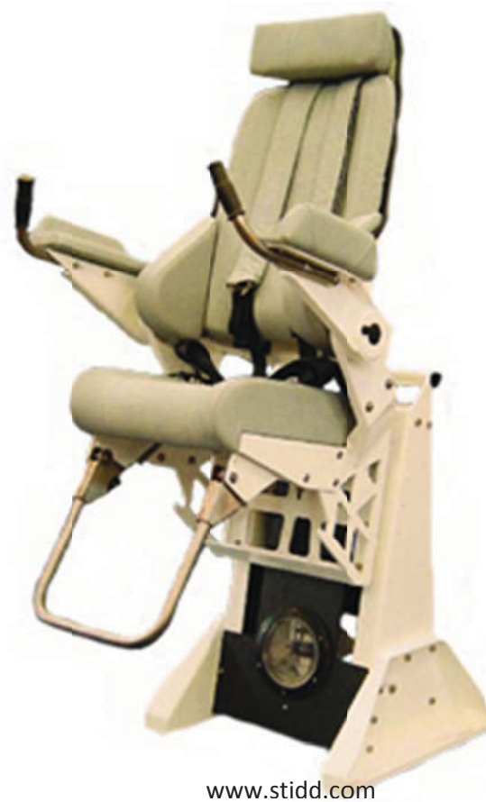
Figure 3-5. Stidd 800v5 shock mitigating seat
