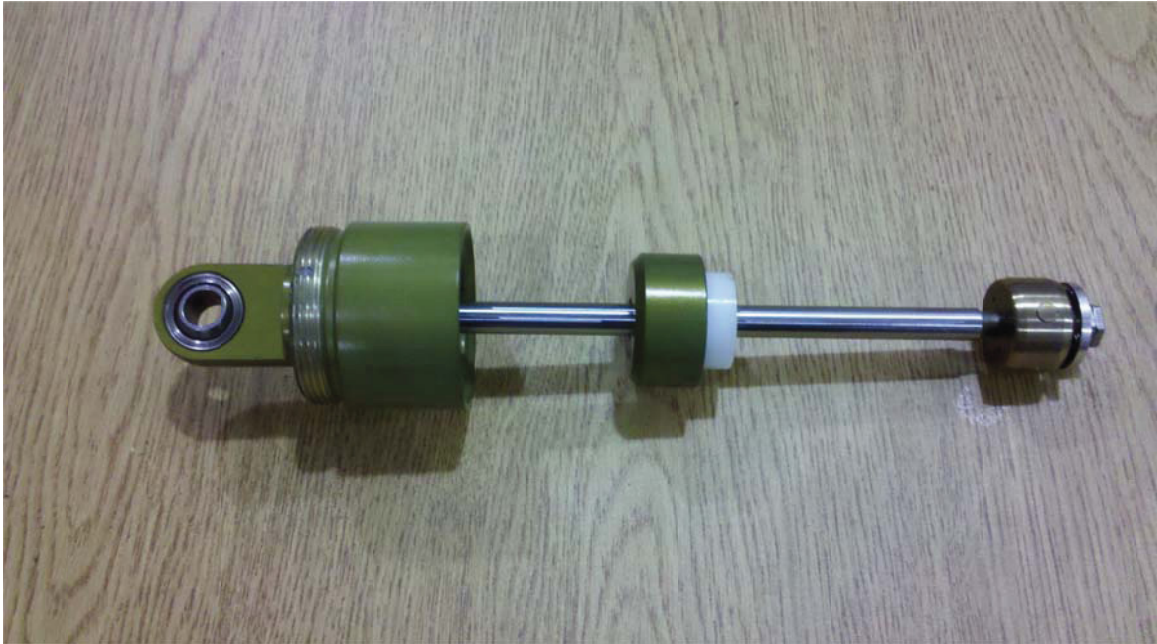
Figure 3-7. Rod and piston assembly removed from shock cylinder.
