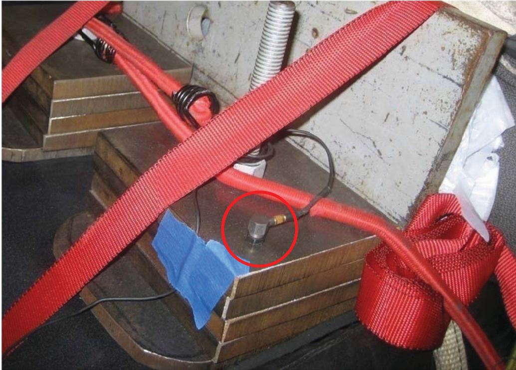
Figure 4-9. Shear accelerometer, circled in red, mounted on top of the occupant mass weights
