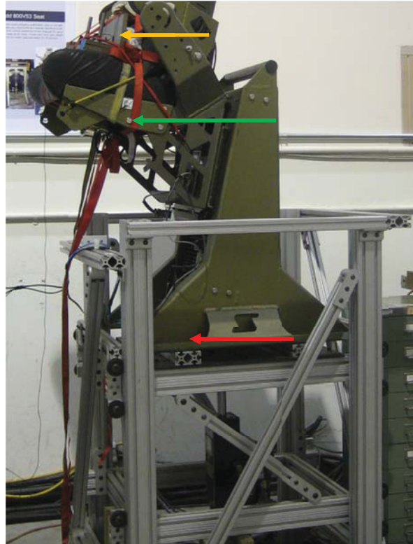
Figure 4-14. Seat Tester with indications of the positions of dynamic measurements. The red arrow represents the base(1), the green arrow represents the seat pan(2) and the yellow arrow represents the mass(3)
