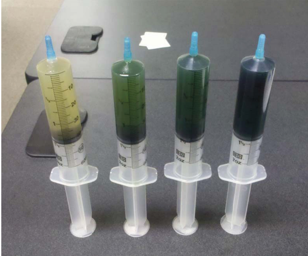
Figure 3-10. Viscosity test setup with equal amounts of fluid in each syringe and same air bubble volume
