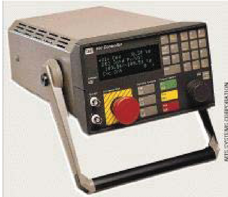
Figure 4-4. MTS 407 Controller used to control the displacement of the MTS 242 actuator
