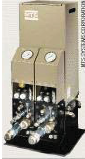
Figure 4-6. MTS hydraulic service manifold used to regulate fluid pressure and flow
