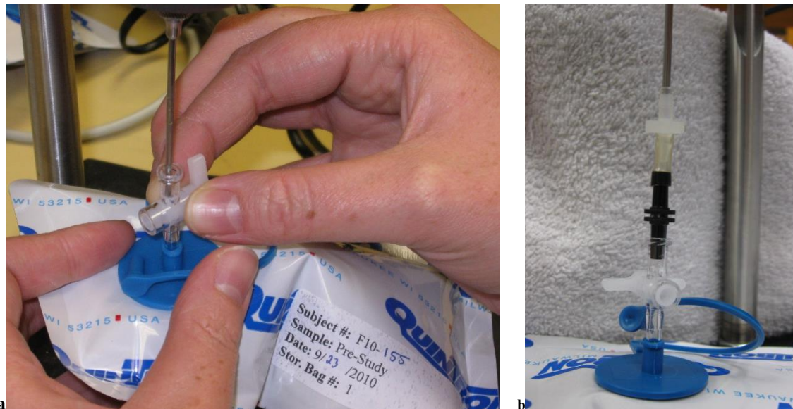
Figure 1. The C320 analyzed breath samples by inserting the snout directly into the storage bag stopcock (a) or by connecting the snout to the storage bag through a series of tubes (b).
