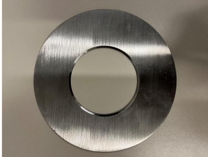
(b) Calibrated Orifice from USA Industries 152.4 mm ID pipe size,  $\beta = 0.5$
