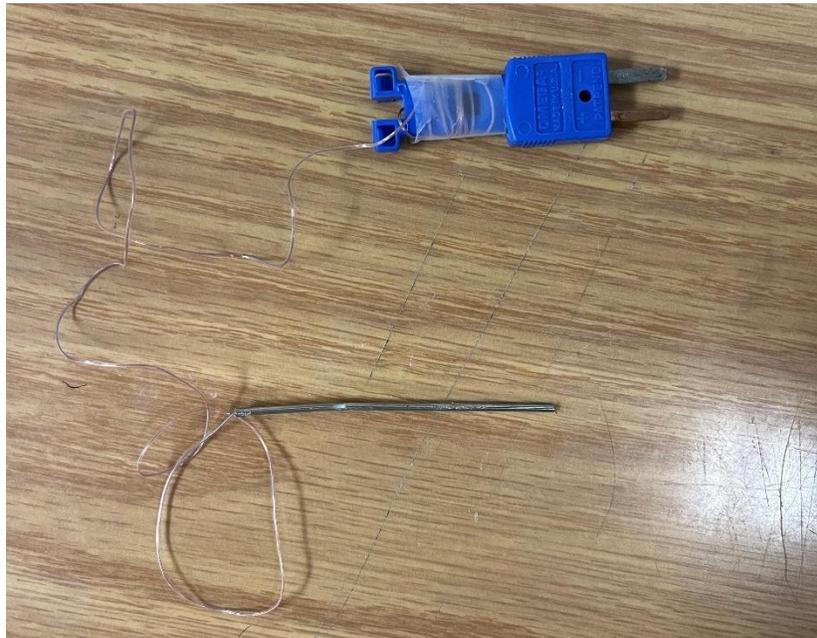
Figure 3-12 Omega T-type Thermocouples
