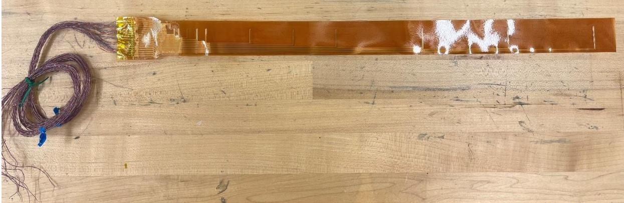
Figure 3-13 FluxTech Thin Film Thermocouple
