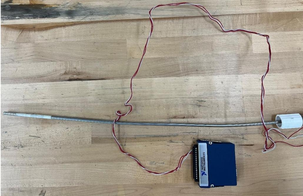
Figure 3-14 Omega PT100 RTD Probe
