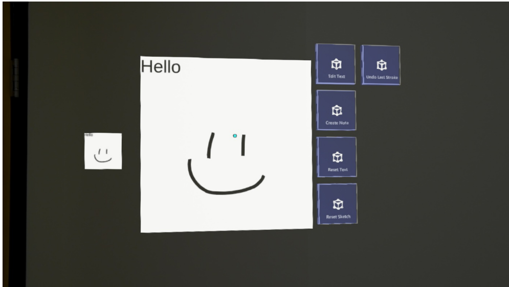
Figure 5.1: An example of our baseline input method. The buttons on the right of the board can be utilized with the Air-Tap gesture. When Create Note is pressed, a virtual note object is generated in front of the user, shown on the left in this figure.
