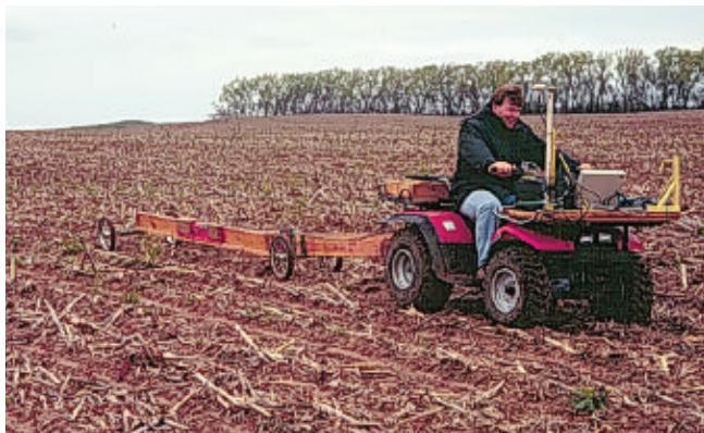
Figure 4. The EM device mounted on a custom-made cart constructed of nonmetallic materials.
