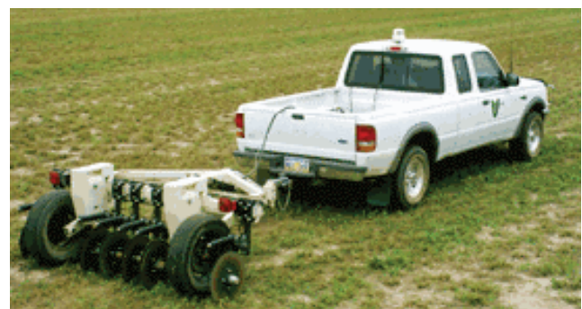
Figure 2. Truck pulling a contact type EC measurement cart in field. Note the DGPS system mounted on the cab to determine the location for the soil EC measurement. (Veris Technologies, Salina, Kansas)
