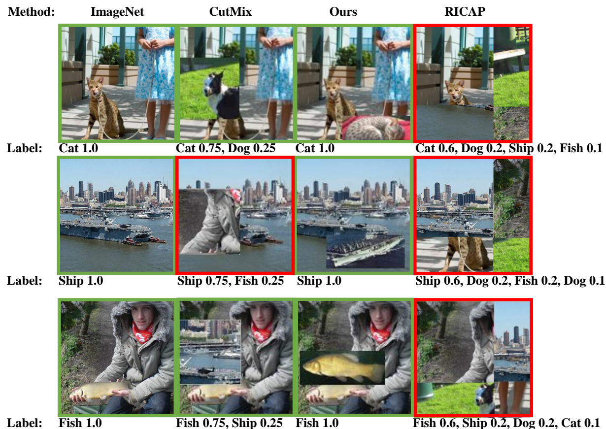
Figure 3.3: We show the differences in recent augmentation methods and the corresponding labels for images generated using the different approaches. Because CutMix and RICAP have no localization information, they are more likely to assign the wrong label to a given crop (red bordered images indicate wrong labels and green bordered images indicate the correct labels), whereas our approach generates correct labels all the time. ImageNet column shows the standard images from the dataset without any augmentation so the labels are not changed during training like the other methods. (Note: The border colors are purely for illustrative purposes. The CNN does NOT receive the samples with the colored borders.)
