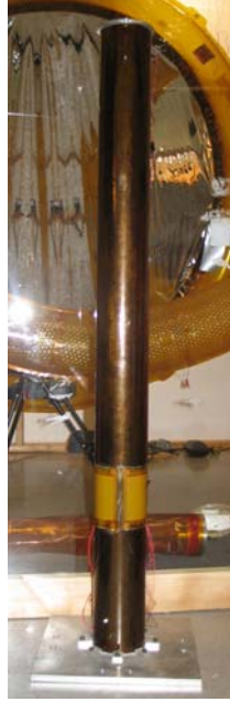
Figure 3-1 An inflatable rigidized boom
