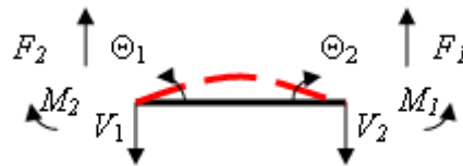
Figure 4-3 Deflection components of a member in bending
