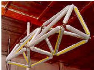
Figure 1-2 A schematic of an inflatable truss element
