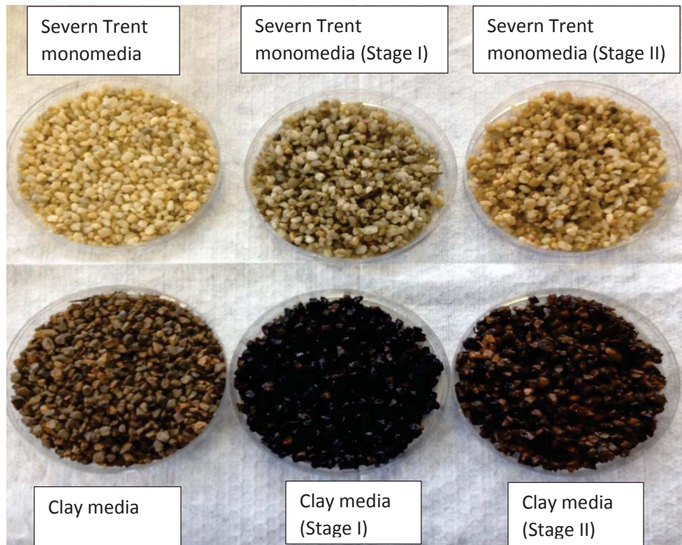
Figure 3.11 Biomass growth on BAF media observed after one month of operation at the PFWTP
