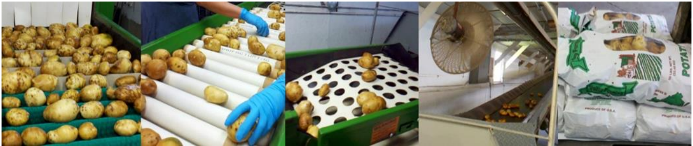
Figure 5. Potatoes running through a packing line system. From left to right: potatoes moving on a conveyer roller after they have been washed under a single-pass spray bar, where they are then sorted by hand to remove poor quality potatoes, and then passed over grading sizer holes to separate out smaller potatoes, then conveyed up a belt where the potatoes are air dried with large fans, and then moved through a chute (not shown) where they are bagged with an automated bagging system. (Amber Vallotton, Virginia Cooperative Extension)
