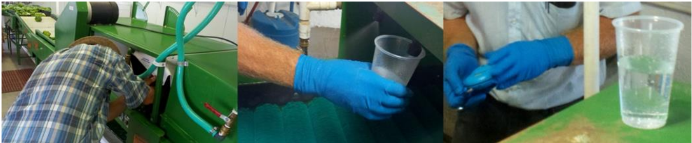
Figure 6. Wash water that has been dosed with chlorine is being sampled from single-pass spray bar nozzles to determine chlorine concentration and pH. (Amber Vallotton, Virginia Cooperative Extension)
