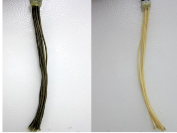
Figure B3 Hollow-fiber membranes before (left) and after (right) chemical cleaning (day 202).
