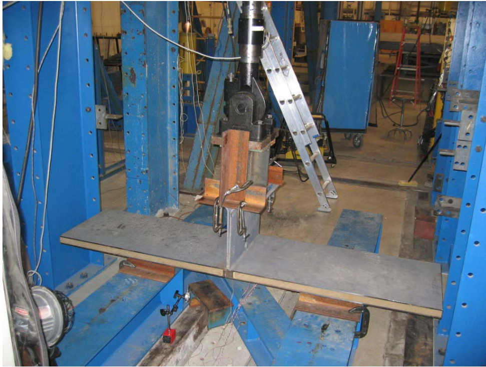
FIGURE 3.9: 5 MILLION CYCLES FATIGUE TEST SETUP
