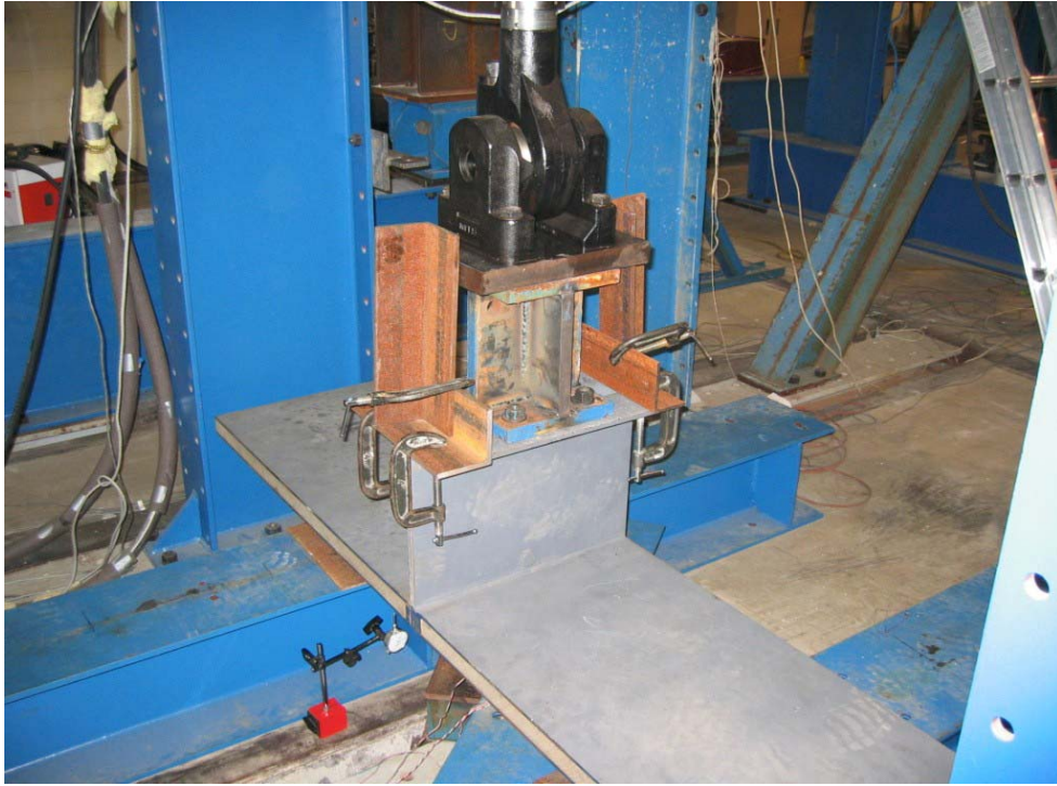
FIGURE 3.10: LOAD BLOCK AND STABILIZING ANGLES
