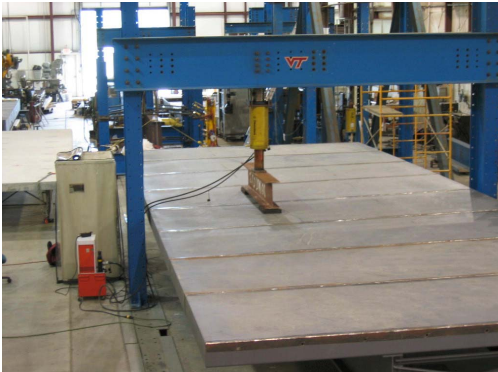
FIGURE D.1: TEST SPECIMEN UNDER MAXIMUM LOADING - UNWELDED PANEL TEST
