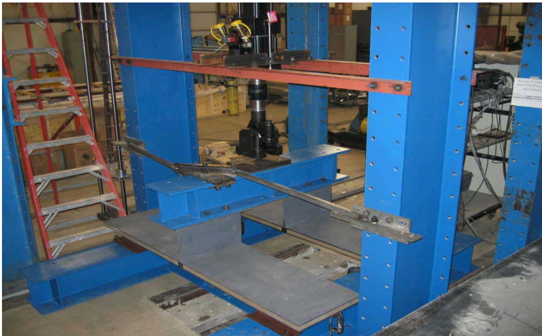
FIGURE 3.5: TEST SETUP FOR CONNECTIONS TESTED TO 10 MILLION CYCLES
