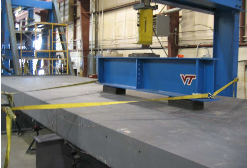
FIGURE 2.17: SANDWICH PLATE BRIDGE DECK AFTER TEST P1-A
