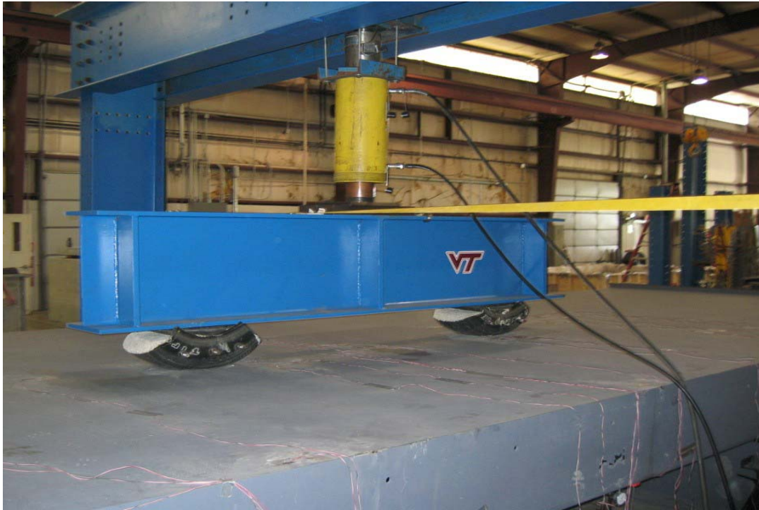
FIGURE 2.9: TEST SPECIMEN UNDER MAXIMUM LOADING - ELASTIC TEST E1-B
