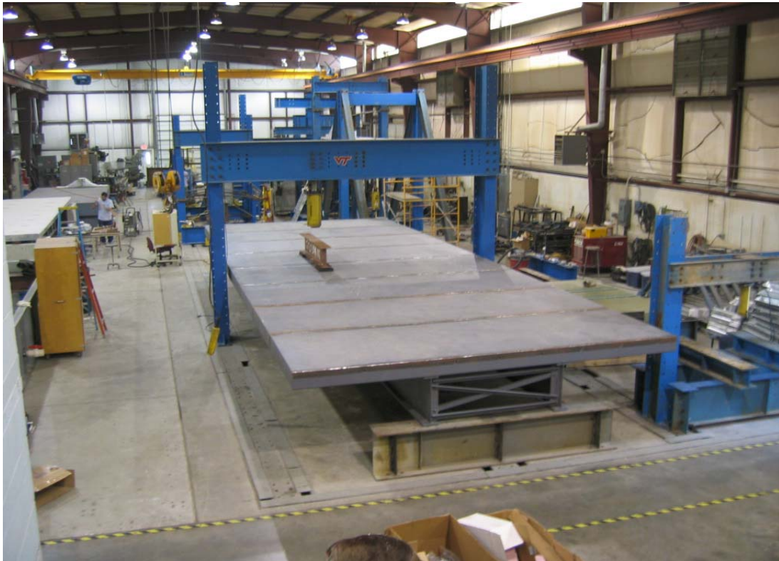
FIGURE 4.2: HALF SCALE CONTINUOUS BRIDGE DECK TEST SPECIMEN
