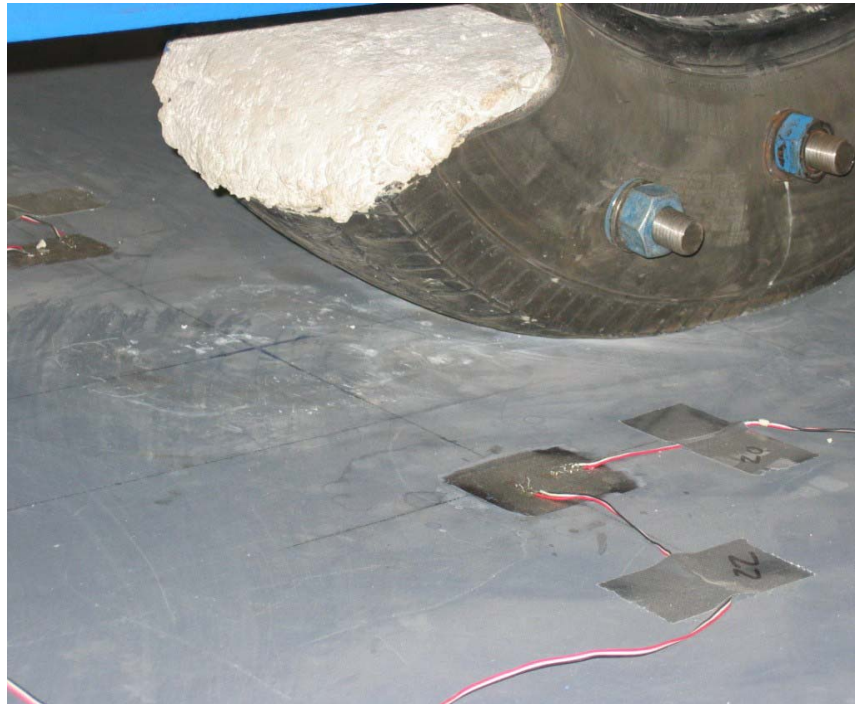
FIGURE 2.3: TIRE LOAD PATCH USED IN ELASTIC TEST E1-A AND E1-B
