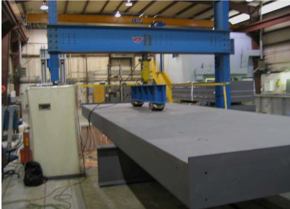
FIGURE 2.5: TEST SPECIMEN UNDER MAXIMUM LOADING - ELASTIC TEST E1-A
