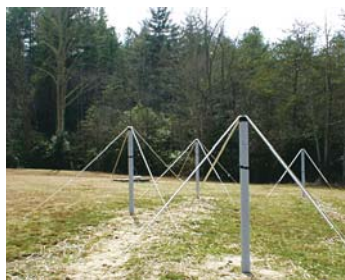
Almost belying its galactic promise, ETA is a visual surprise: it looks like 12 pipes stuck in the grass at the Pisgah Astronomical Research Institute (PARI) near Asheville, N.C. Each stand, however, is a carefully situated, dual-polarized, 38-MHz-resonant dipole antenna, individually instrumented and digitized. The complete array continually scans the entire sky using fixed “patrol beams.”
