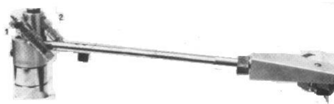
Figure 4: Tension and Compression Spring Equilibrated Record Player Arm
