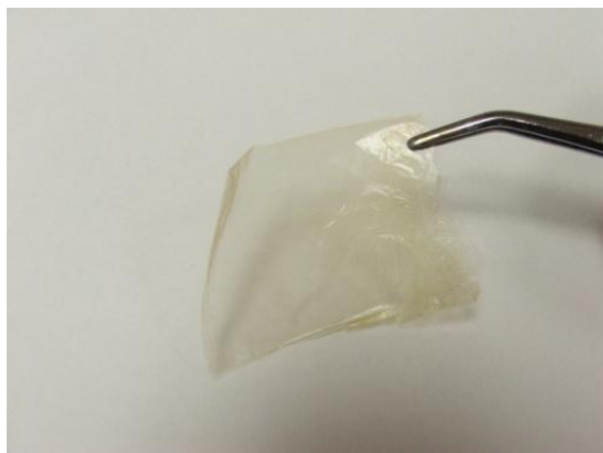
Figure 5. 11 A free-standing film of NC-PDDA-HMWL obtained after 250 deposition cycles. The free-standing films were obtained after dissolving the cellulose acetate substrate in acetone.
