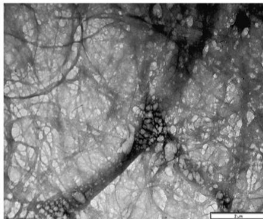
Figure 2. 11 Transmission electron micrograph of microfibrillated cellulose (Lu, J.; Askeland, P.; Drzal, L. T., Polymer 2008, 49, 1285-1296, used under the fair use guidelines, 2011).
