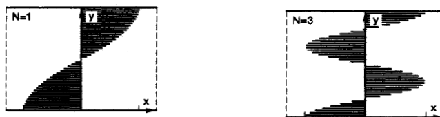
Figure 2. 18 Shear displacement profiles across the quartz crystal thickness for the fundamental and third overtone (Martin, S. J.; Granstaff, V. E.; Frye, G. C., Anal. Chem. 1991, 63, 2272-228, used under the fair use guidelines, 2011).
