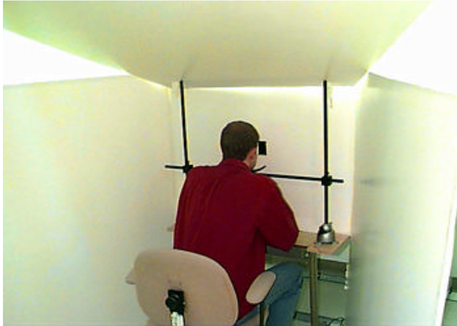
Figure 7. Viewing-booth/light-chamber used to control glare in experiment.
