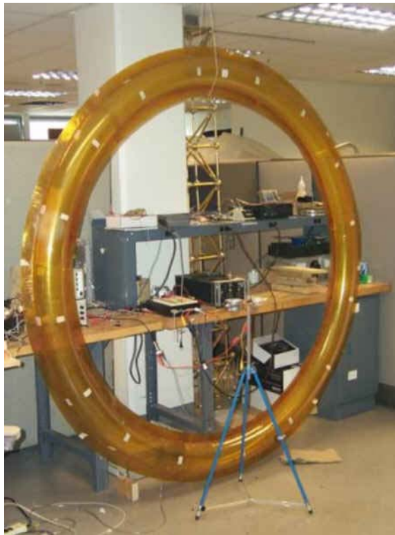
Figure 3.2: Inflated torus suspended in free-free boundary conditions.
