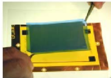
b) Placement of fiber sheet on electrode film.
