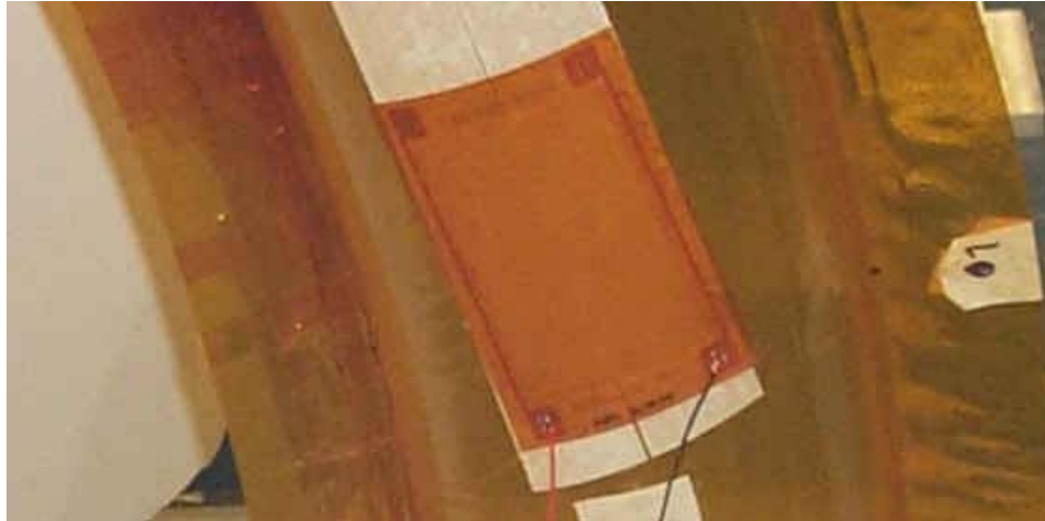
Figure 3.3: Macro-fiber composite bonded to the torus.
