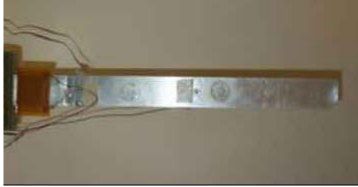
Figure 2.8: Picture of MFC bonded to aluminum beam.
