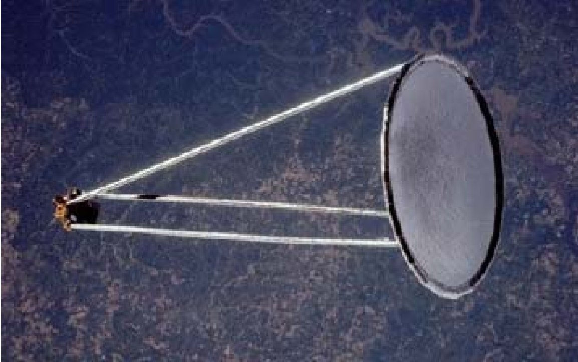
Figure 1.10: Spartan 207/Inflatable Antenna Experiment in orbit (Figure from NASA).
