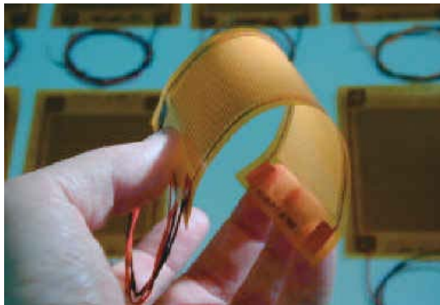
Figure 3.1: Macro-fiber composite being bent to show its flexibility.
