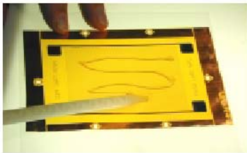
a) Preparation of bottom electrode film with epoxy adhesive.
