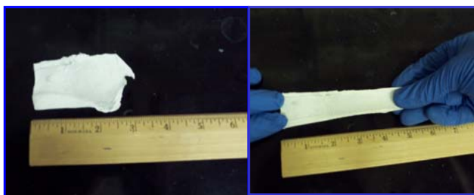
Non-woven highly branched PUU mats exhibit elastomeric behavior.
