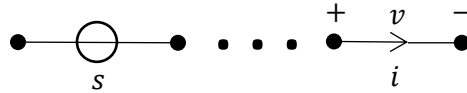
Figure 4: Voltage and Current conventions for GTA model, where S is the reference source f
