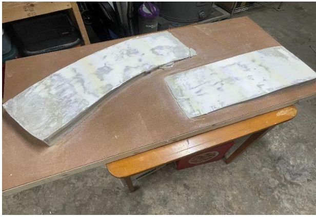
Cast concrete ramp apparatus
