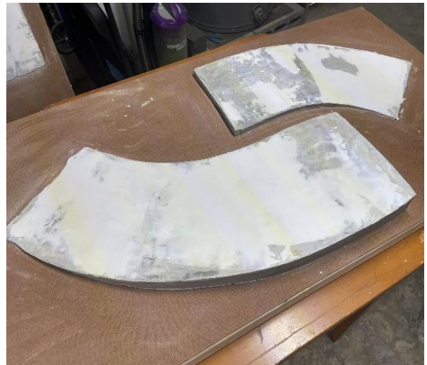
Cast concrete ramp apparatus
