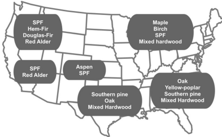
Figure 1: Wood species common to each region of the United States (adapted from Park 2015).
