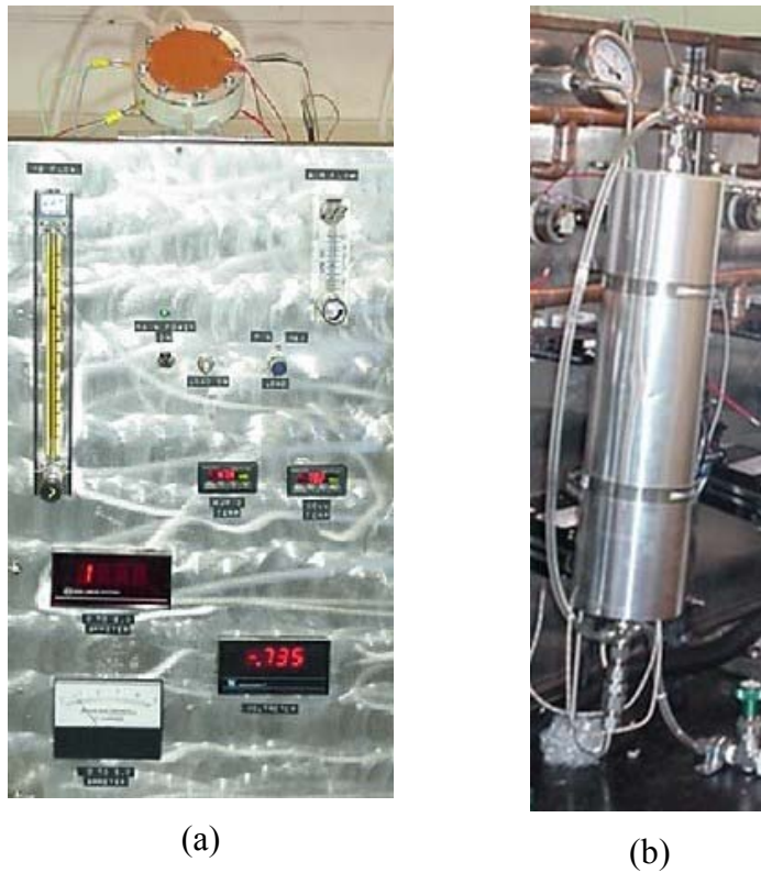
Figure 3-4: (a) An individual test station, and (b) cathode humidifier.
