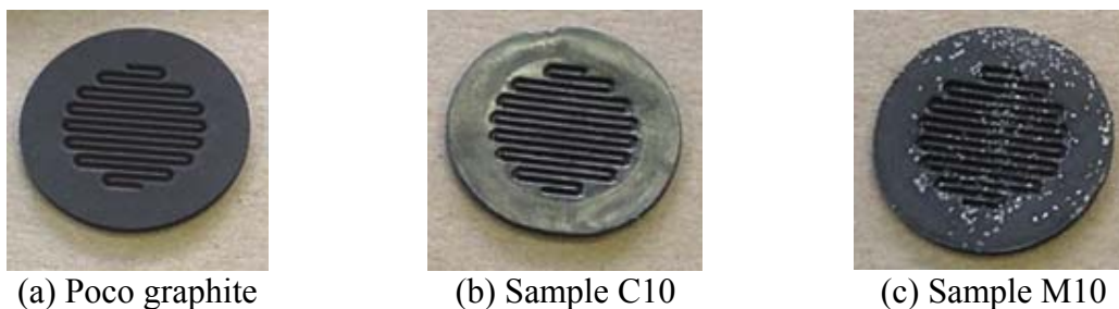
Figure 4-3: Photos of (a) Poco graphite, (b) C10, and (c) M10 monopolar plates.
