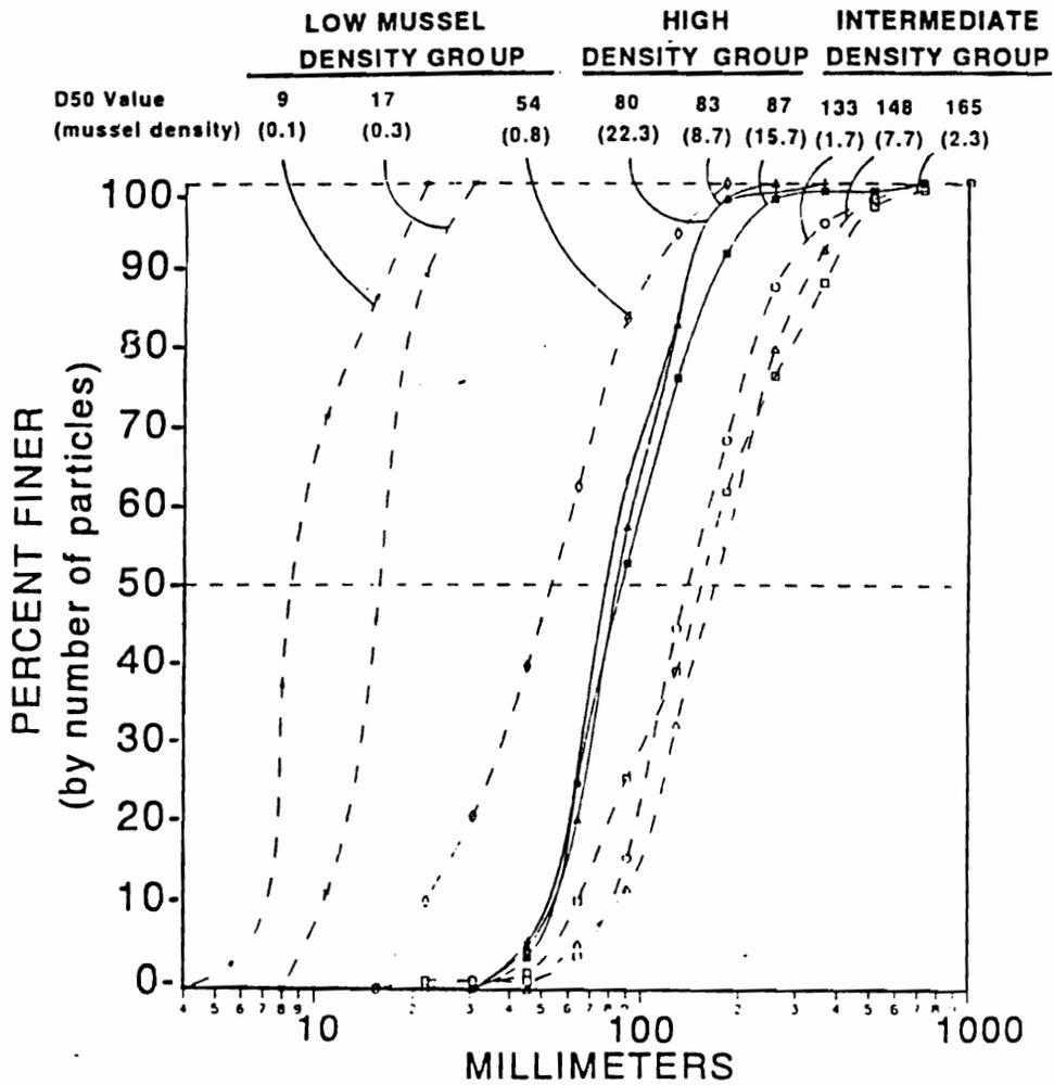
Figure A.4. Particle size distribution curves for nine Little River transects. Note that the high mussel density group (solid lines) occurs in a particle size range between low and intermediate mussel density groups.
