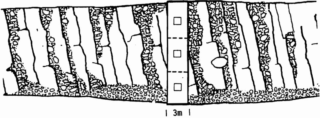
Figure A.2. Mussel density and percent bedrock (PBR) sampling methods. Three 1 m<sup>2</sup> quadrats were excavated in each 3 m wide transect zone. A visual estimate was made of the percent bedrock in each transect zone.
