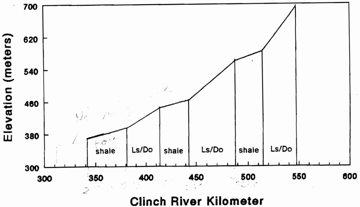
Figure 4.6. Plot of Clinch River kilometers against elevation. Note that limestone/dolomite (Ls/Do) reaches are characterized by higher gradient than shale reaches.
