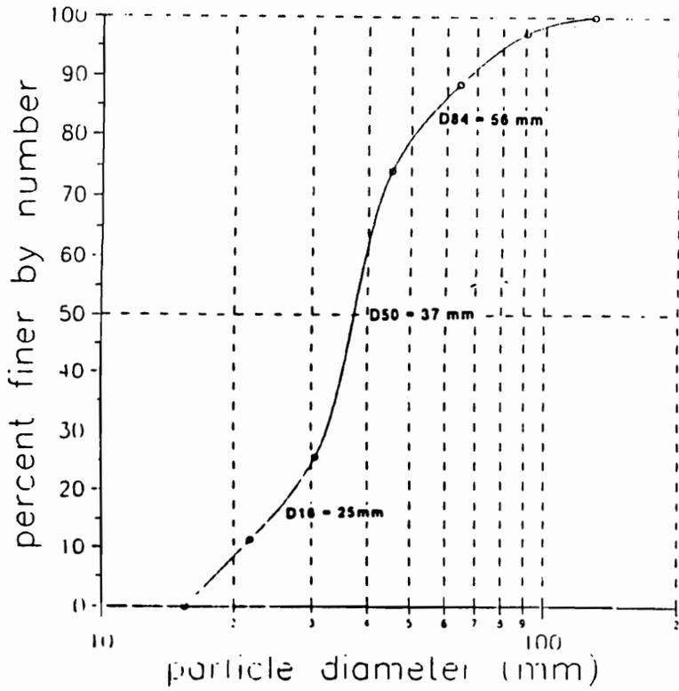
Figure A.3. A sample particle-size distribution curve from the Little River. D50 particle-size is also referred to as median particle size.
