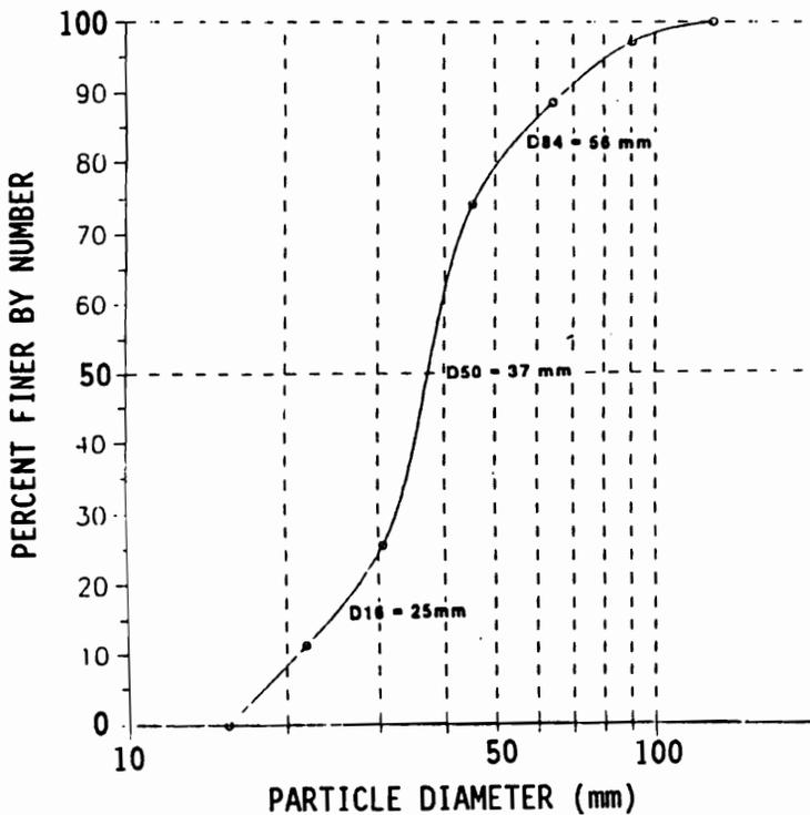
Figure 3.3. Particle-size distribution curve for a streambed sample from the Little River. The d50 particle size is also referred to as the median particle size.
