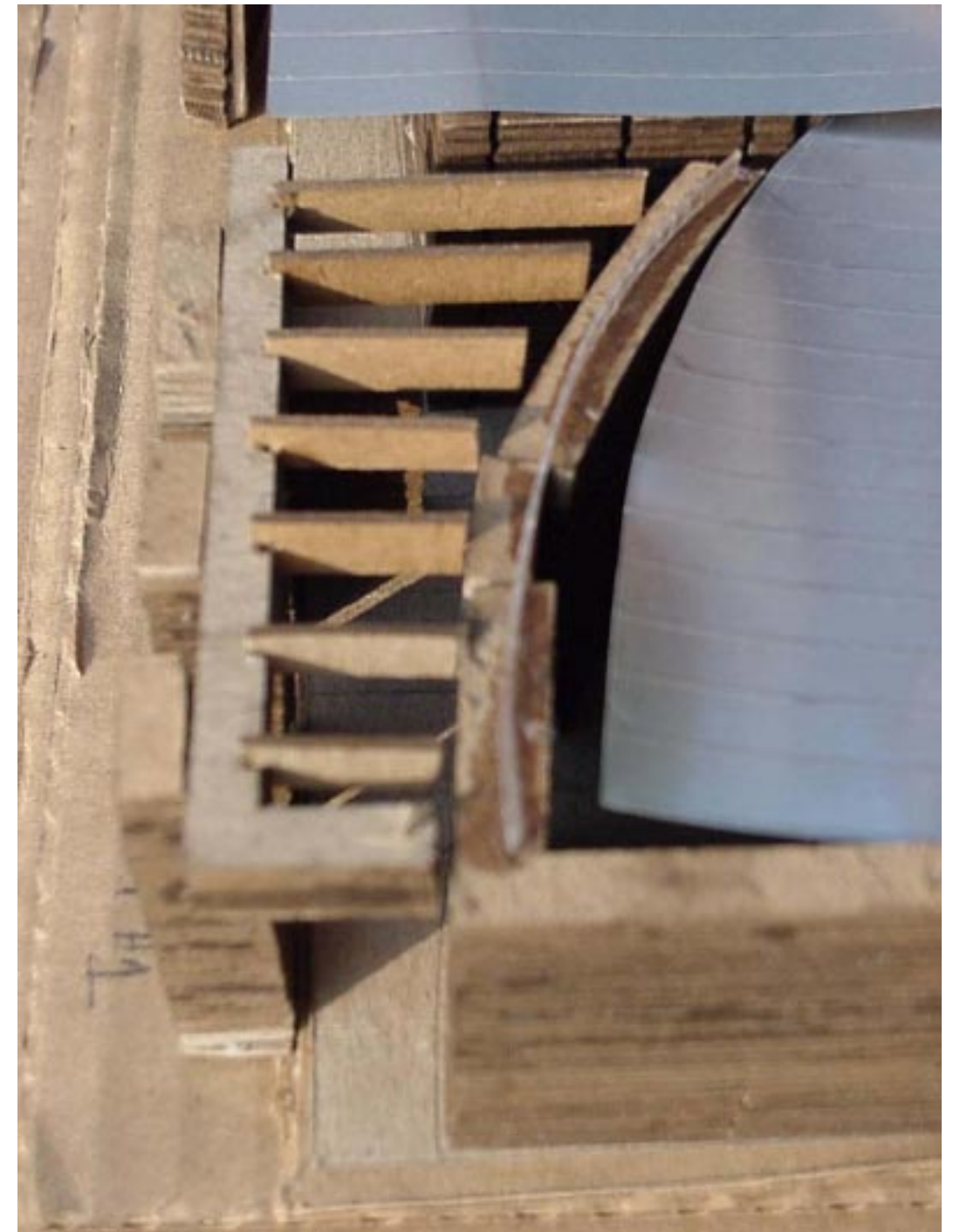
Brise-Soleil over the outdoor gathering place, on the west facing facade.
