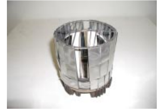
Addition of the steel panels acting as skin.
