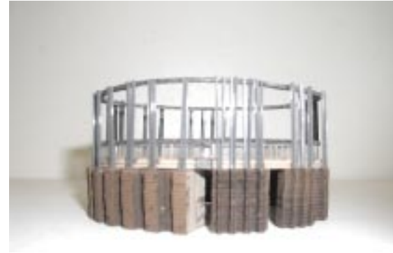
Placement of concentric rings as horizontal support members.
