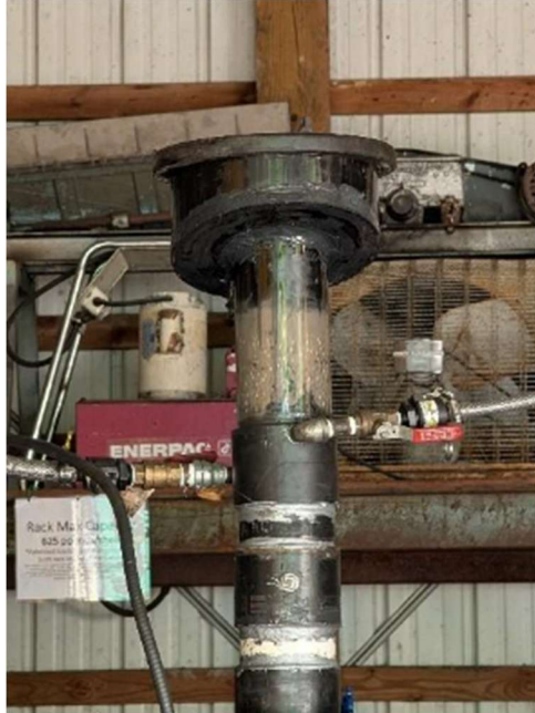
Figure 4.5: Extended Jig Morganizer with visible phase separation.
