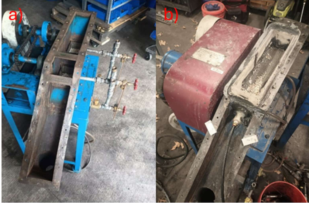
Figure 3.13: Conventional jig modified for Jig Flotation.
