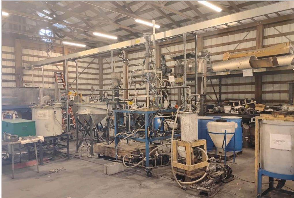
Figure 4.3: Two-Liquid Flotation Process Demonstration Unit.
