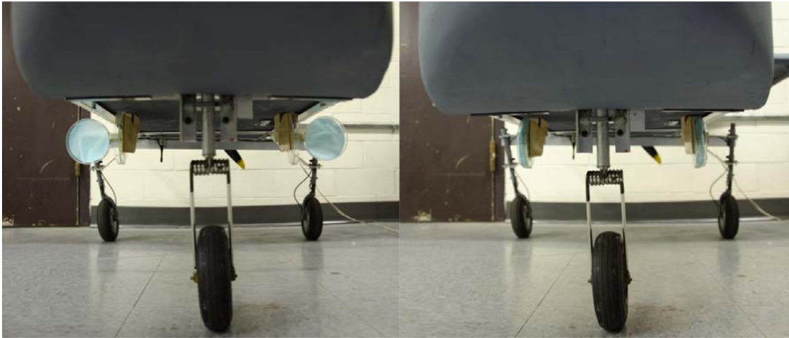
Figure 3.6: Petri plate samplers on the underside of SPAARO open (left) and closed (right). The filter papers can be seen to be blue after capturing blue dye particles in flight. Photos courtesy of Mark C. Palframan.
