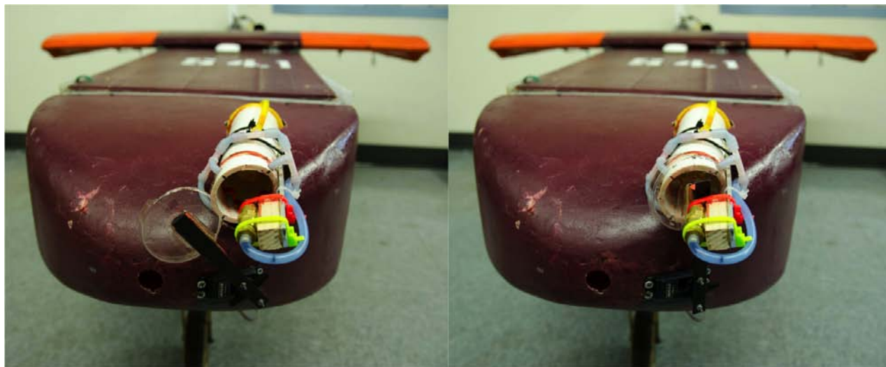
Figure 3.7: The servo operated sampler end cap is shown open for sampling (left) and then closed (right). The misting spray head can also be seen in front of the collection tube opening, while tubing for the recirculating wash mechanism can be seen on the outside of the collection tube. Photos courtesy of Mark C. Palframan.
