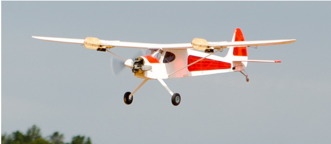
Figure 3.2: A Sig Rascal 110 in flight with closed petri plate samplers seen on the leading edge of each wing. Photo courtesy of Mark C. Palframan.
