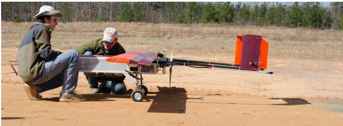
Figure 3.4: The aerial spray system is tested on the ground with a blue dye before flight at Fort Pickett in Blackstone, Virginia. The two spray lines can be seen attached to the underside of the tail booms. Photo courtesy of Mark C. Palframan.
