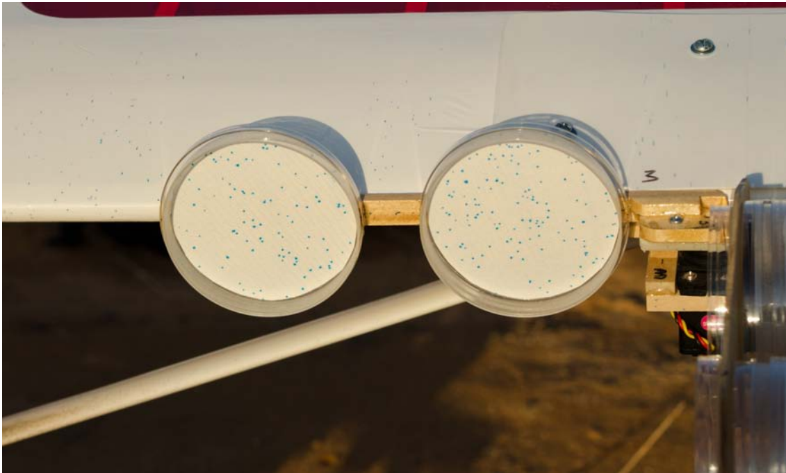
Figure 5.1: A Sig Rascal's airframe with wing mounted filter paper petri samplers was flown behind a SPAARO UAV releasing misted blue dye at Fort Pickett in Blackstone, Virginia. Spots of blue dye were found on the filter paper samples as well as on the leading edge of the wing. Photo courtesy of Mark C. Palframan.
