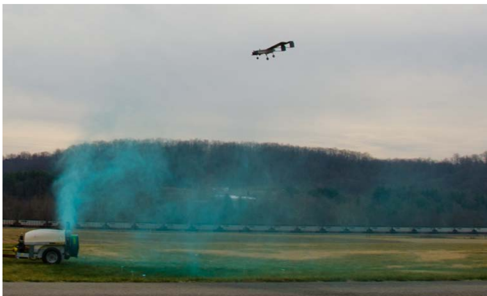
Figure 5.2: SPAARO flew through and collected samples from a plume of dyed water generated by an orchard sprayer at Virginia Tech’s Kentland Farm facility. Photo courtesy of Mark C. Palframan.
