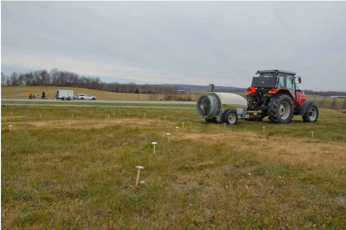
Figure 5.3: An semicircle array of petri dishes containing filter papers was placed around an orchard sprayer. The filter papers collected samples from the orchard sprayer plume which were later used to characterize the plume distribution. Photo courtesy of Mark C. Palframan.
