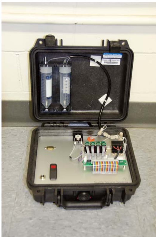
Figure 2.3: The SPIRIT SPR sensor system was originally designed to be used as a rugged mobile field unit. Photo courtesy of Mark C. Palframan.
