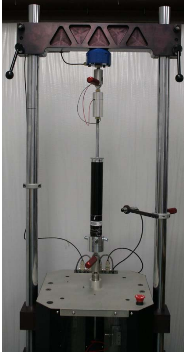
Figure 2.2. Laboratory setup for experimental characterization of the MR damper.
